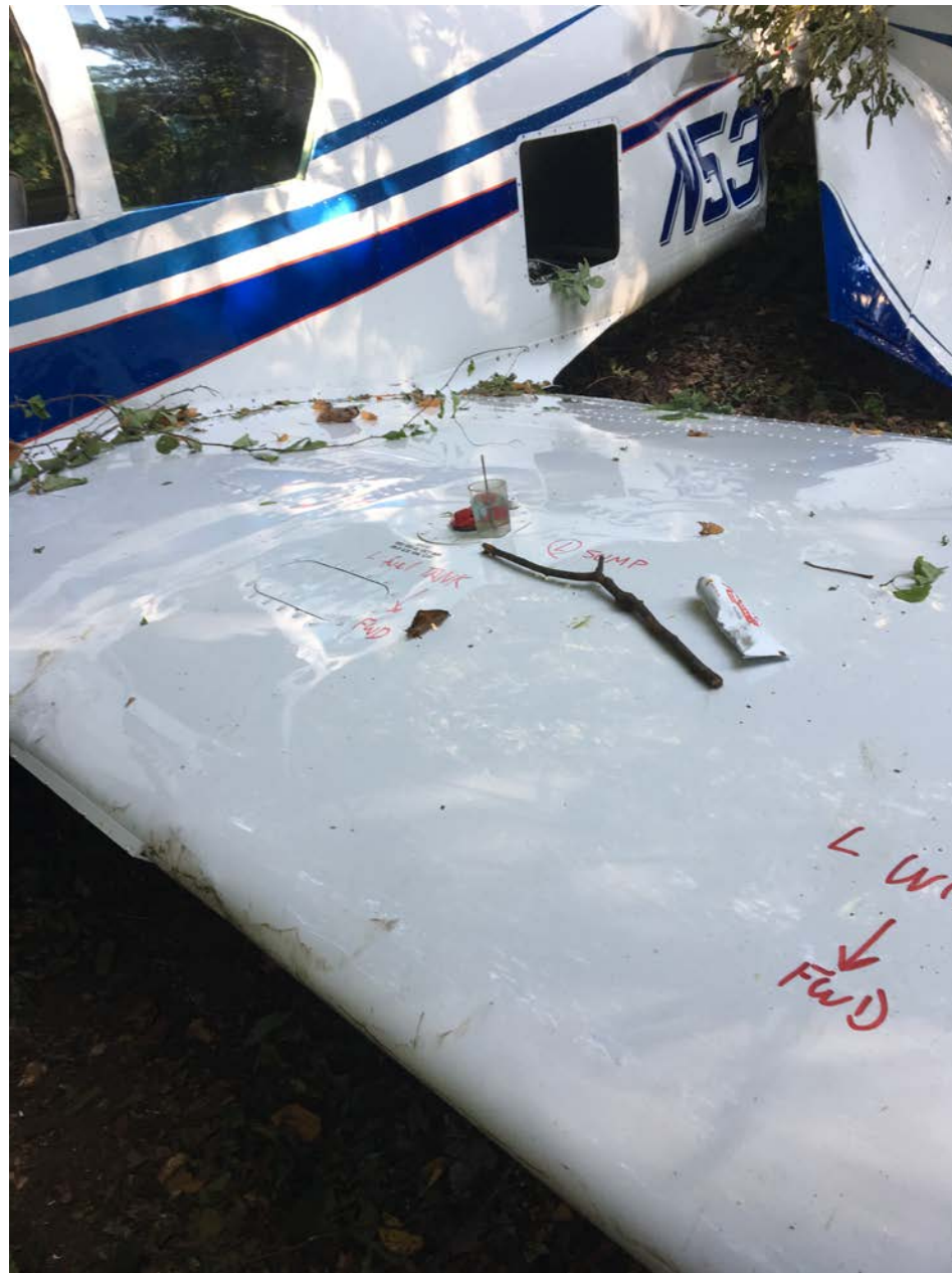
Photo 5 - Left wing leading edge looking towards fuselage. The fuel tank sump tester is full of aviation fuel.
