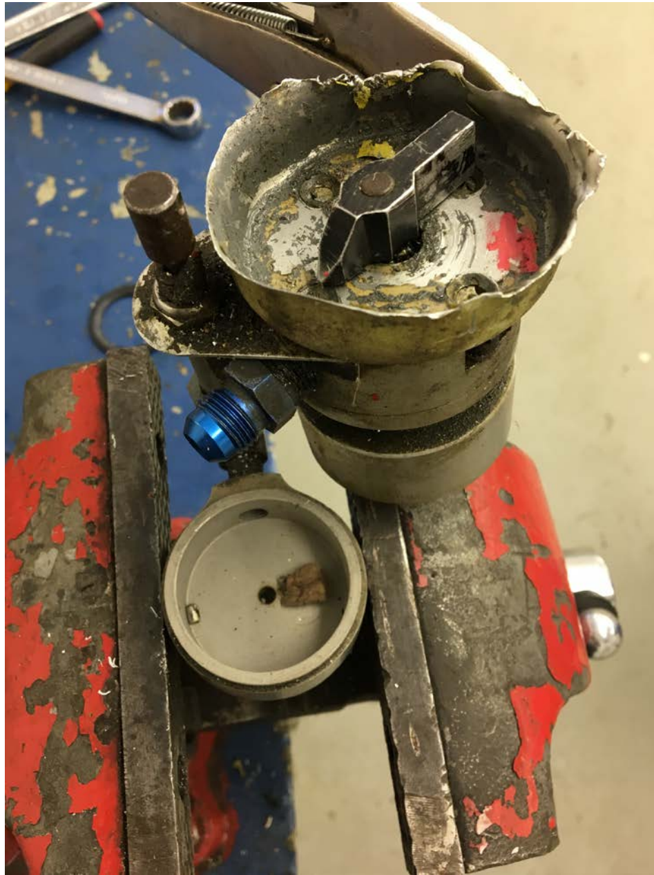
Photo 9 – Fuel selector valve partially disassembled showing fibrous debris in selector cavity.
