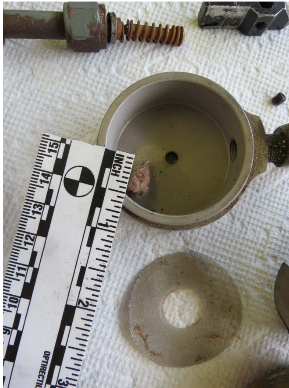
Photo 10 – Close up view of red tinted fibrous material on drain screen and in fuel selector cavity.
