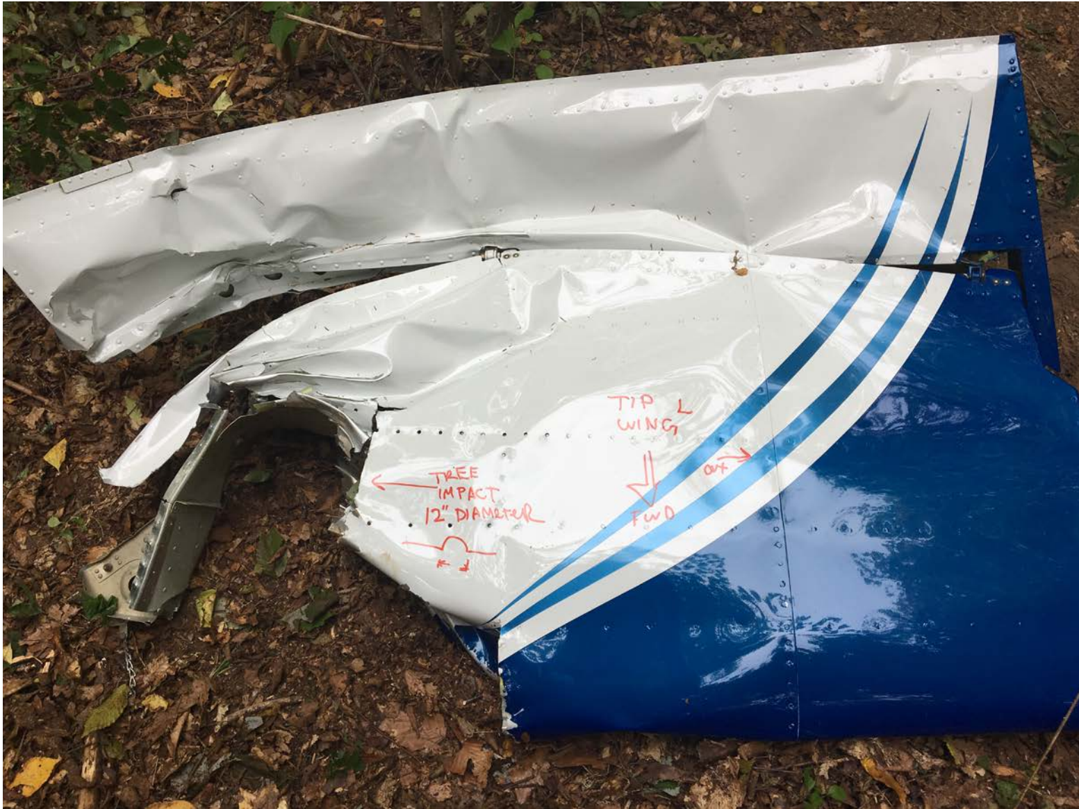
Photo 6 – Separated left wingtip and aileron showing tree impact damage.
