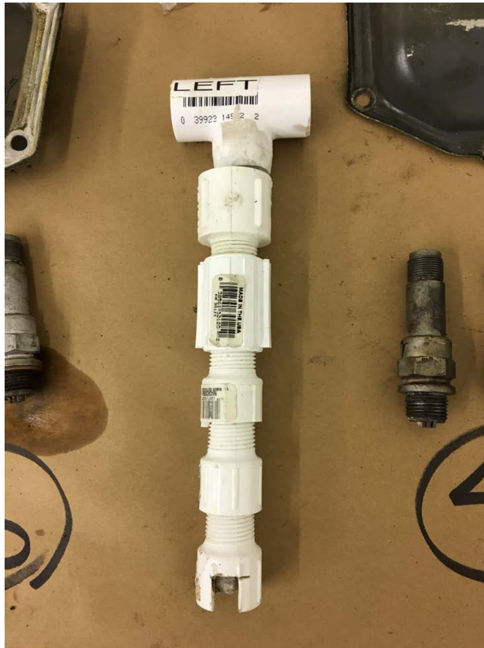
Photo 8 – Photograph of homemade PVC handle used to change the fuel selector. The handle is broken at the top and separated from the bottom attachment.
