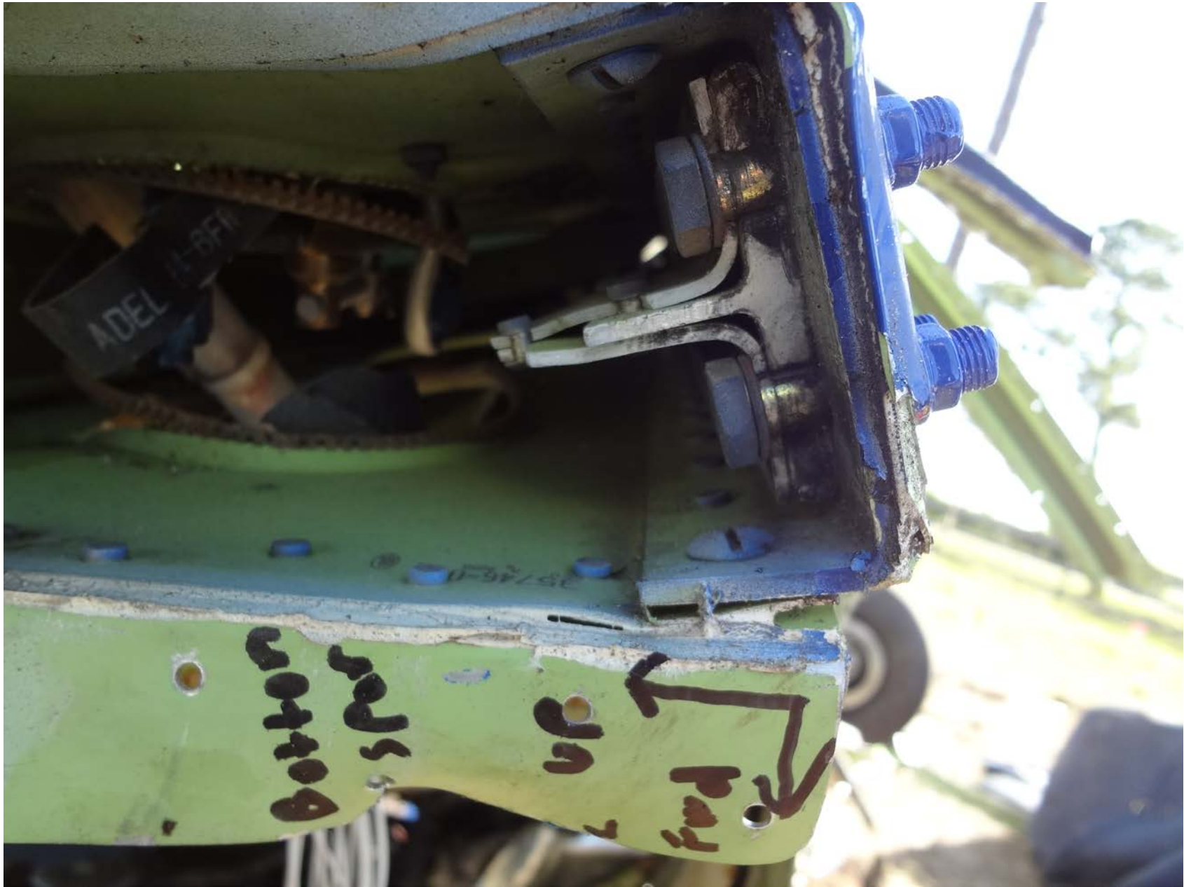
Photo 7 – Close up view of left fuselage wing spar and fracture surface.
