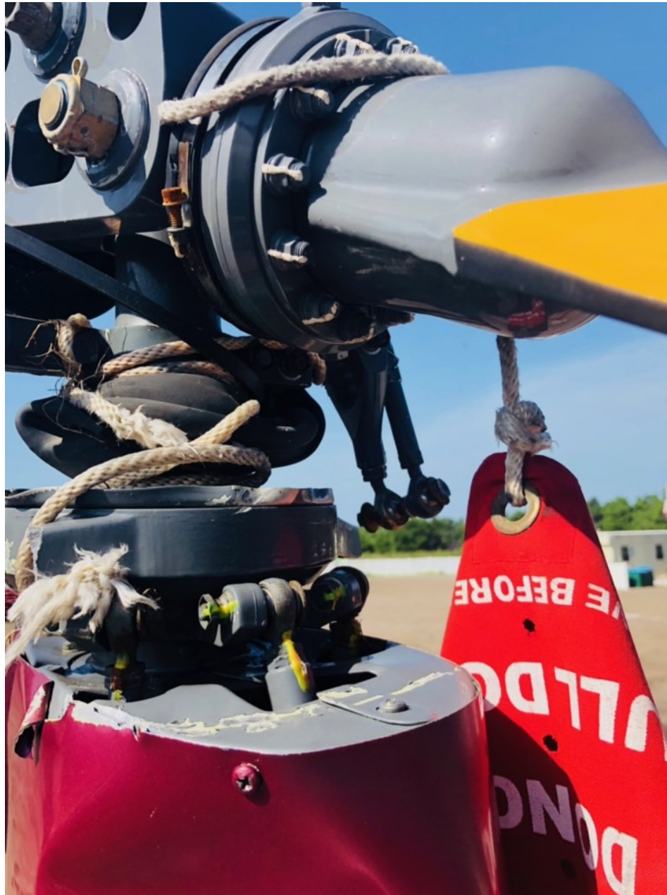
Photo 3 – Close up of damage and rotor blade tie down rope wrapped around rotor assembly.
