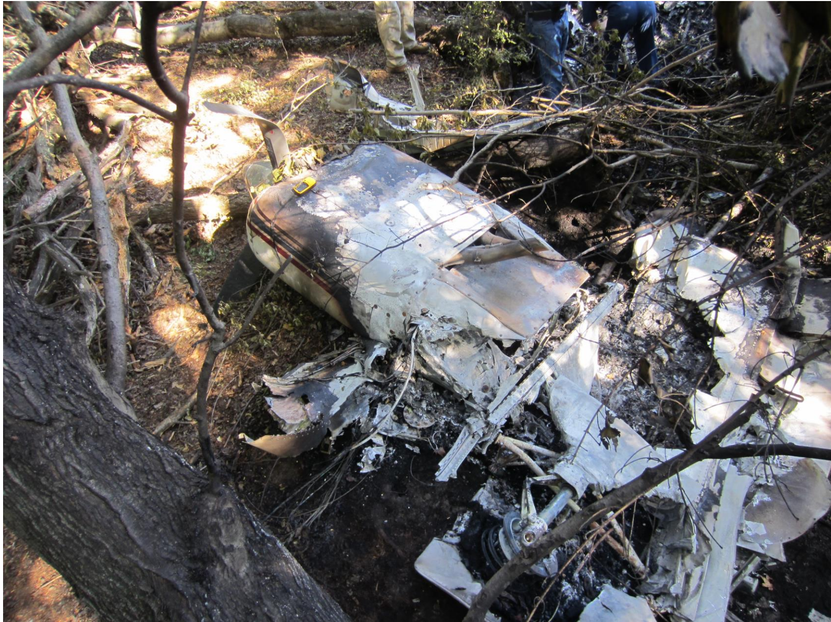
Photo 3 – Left engine, propeller and wing damage. The entire assembly is upside down.
