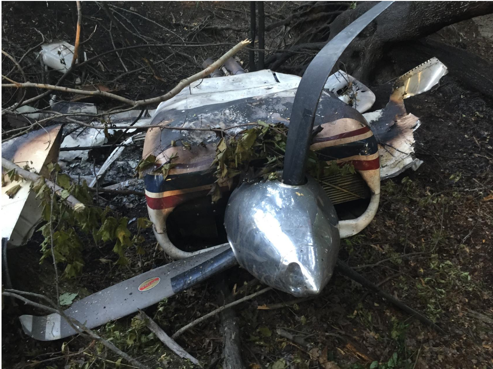
Photo 4 –Close up view of left propeller and engine damage.
