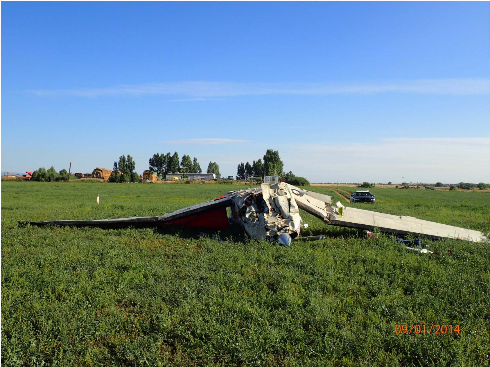
Photo 1 – View of the inverted main wreckage. Photo taken from nose looking aft toward tail.
