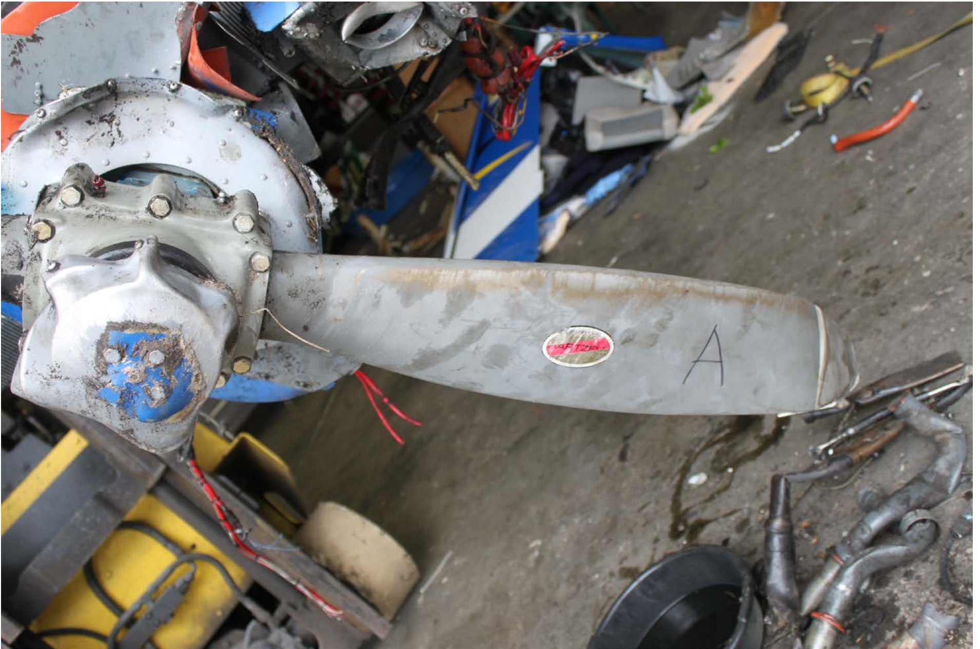
Photo 3 – Damage to Propeller Blade
