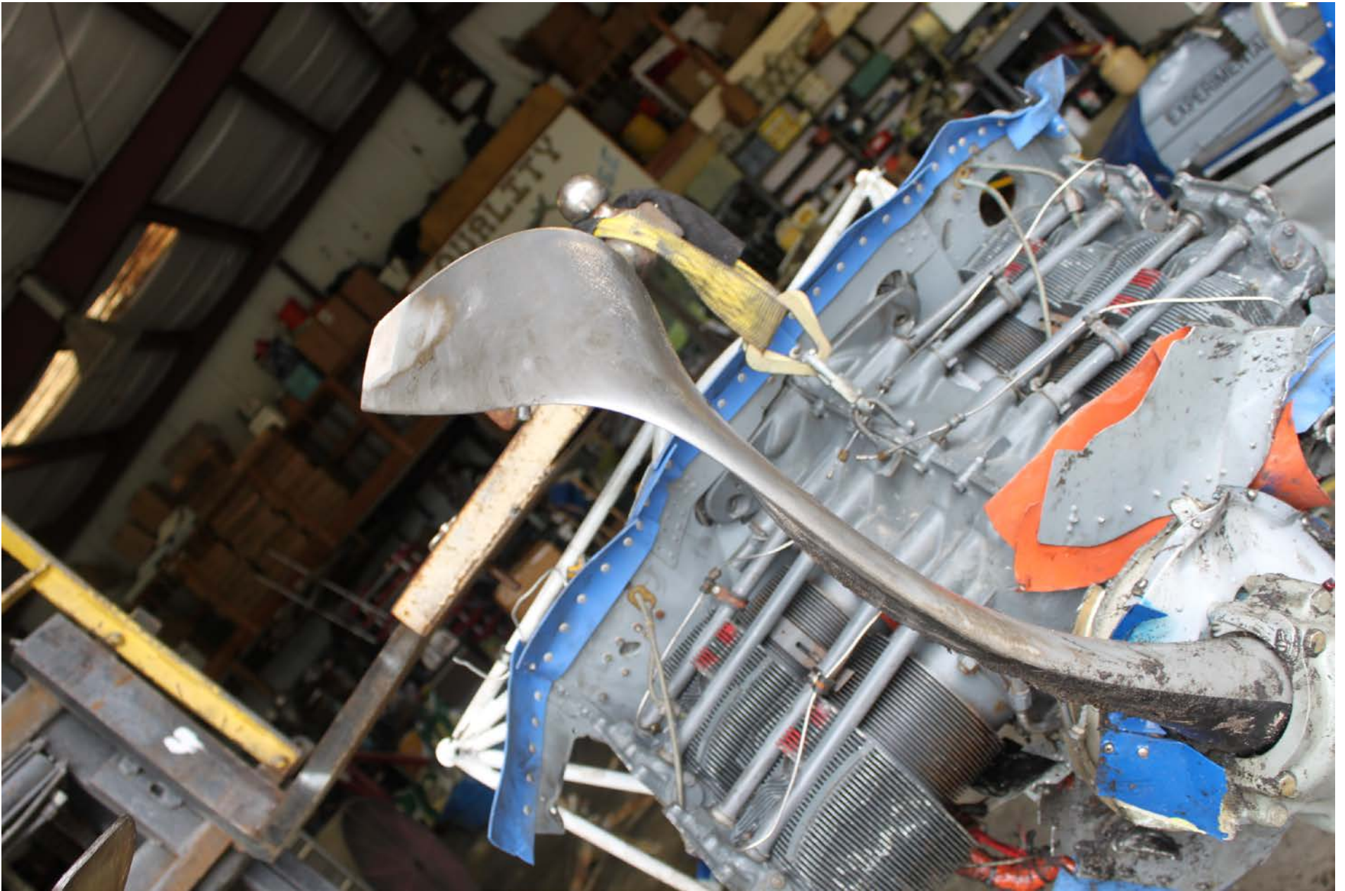
Photo 4 – Damage to Propeller Blade
