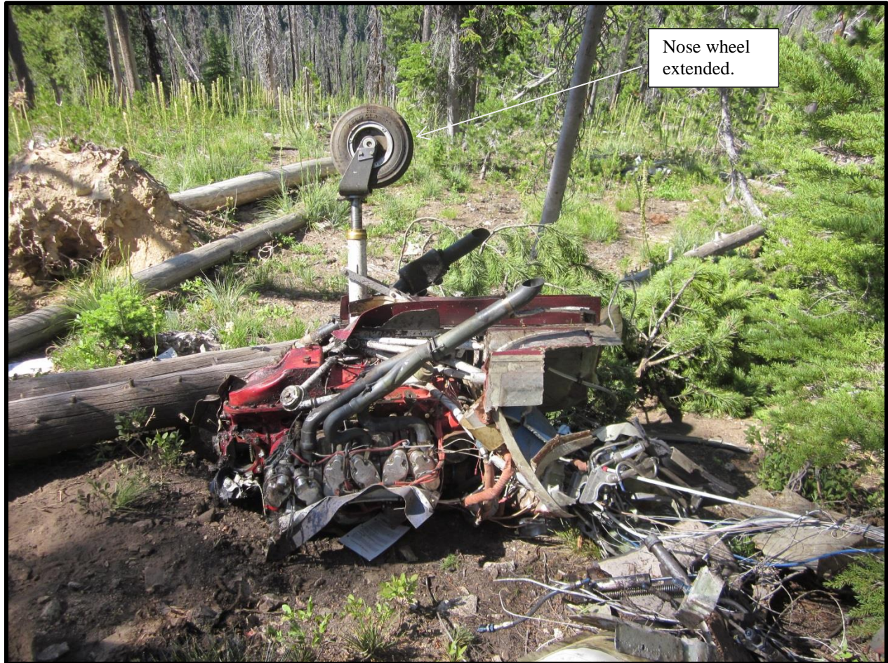
Figure 3: View of Engine Inverted on the Ground.
