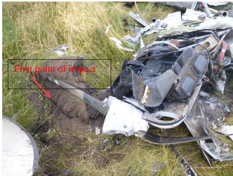
Photo 2. First point of impact
