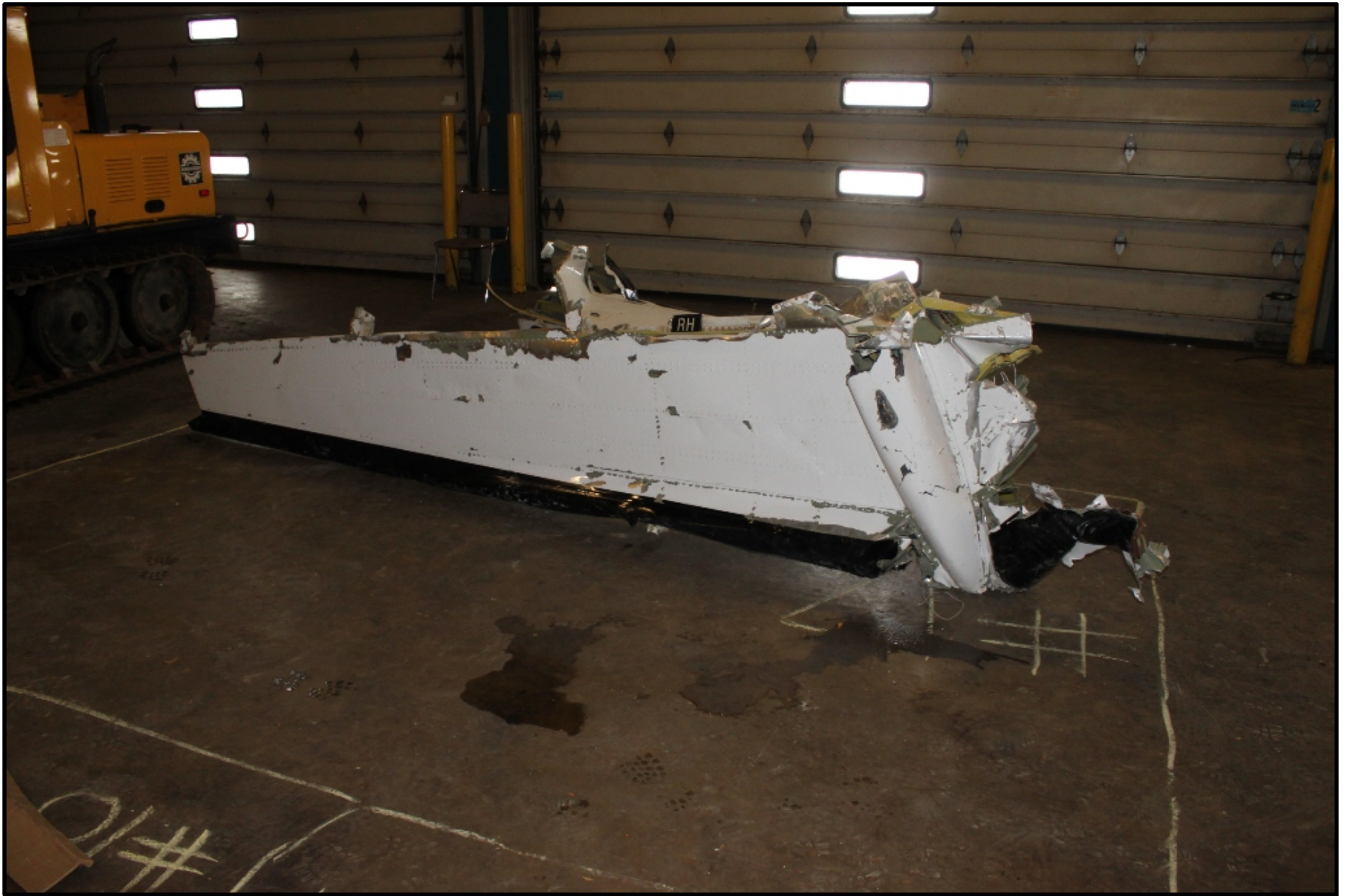
Photo 4 – Right Horizontal Stabilizer
