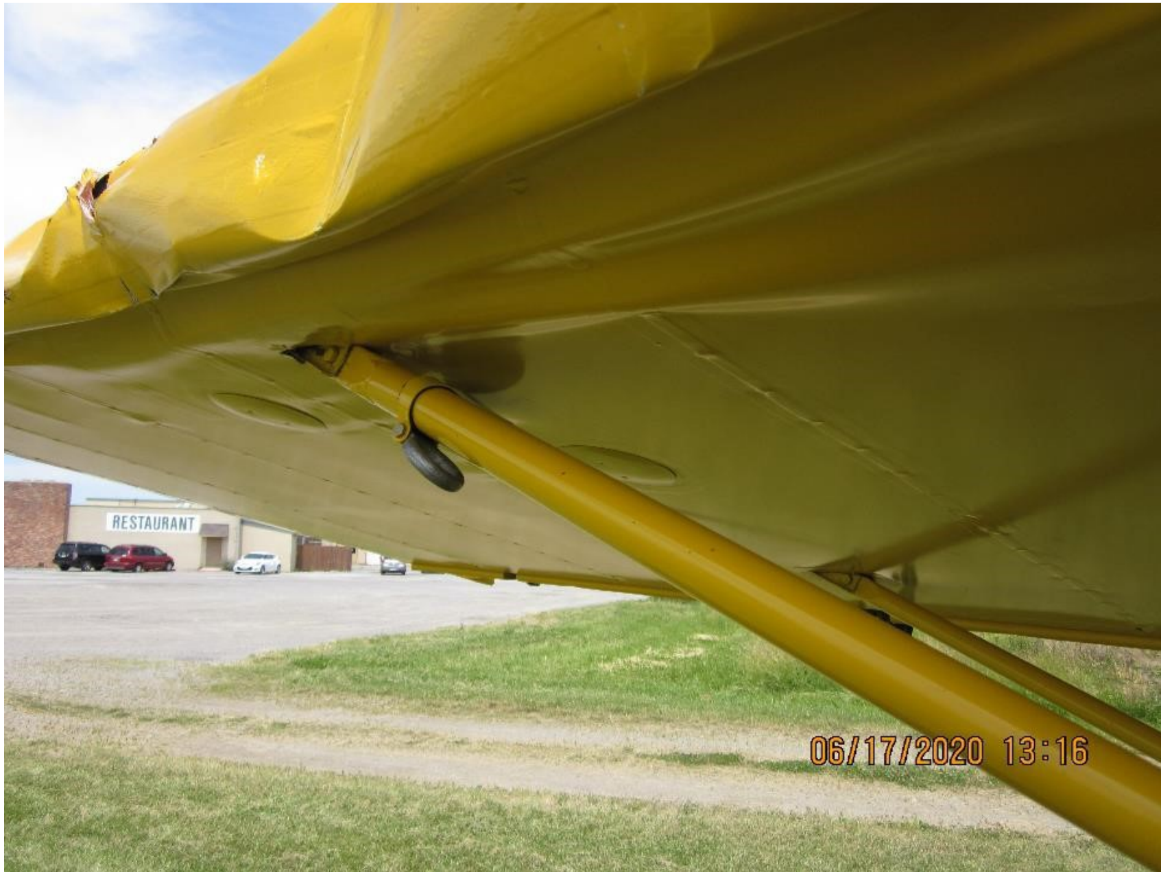
Photo 4 – Another view of right wing leading edge damage (FAA photo)
