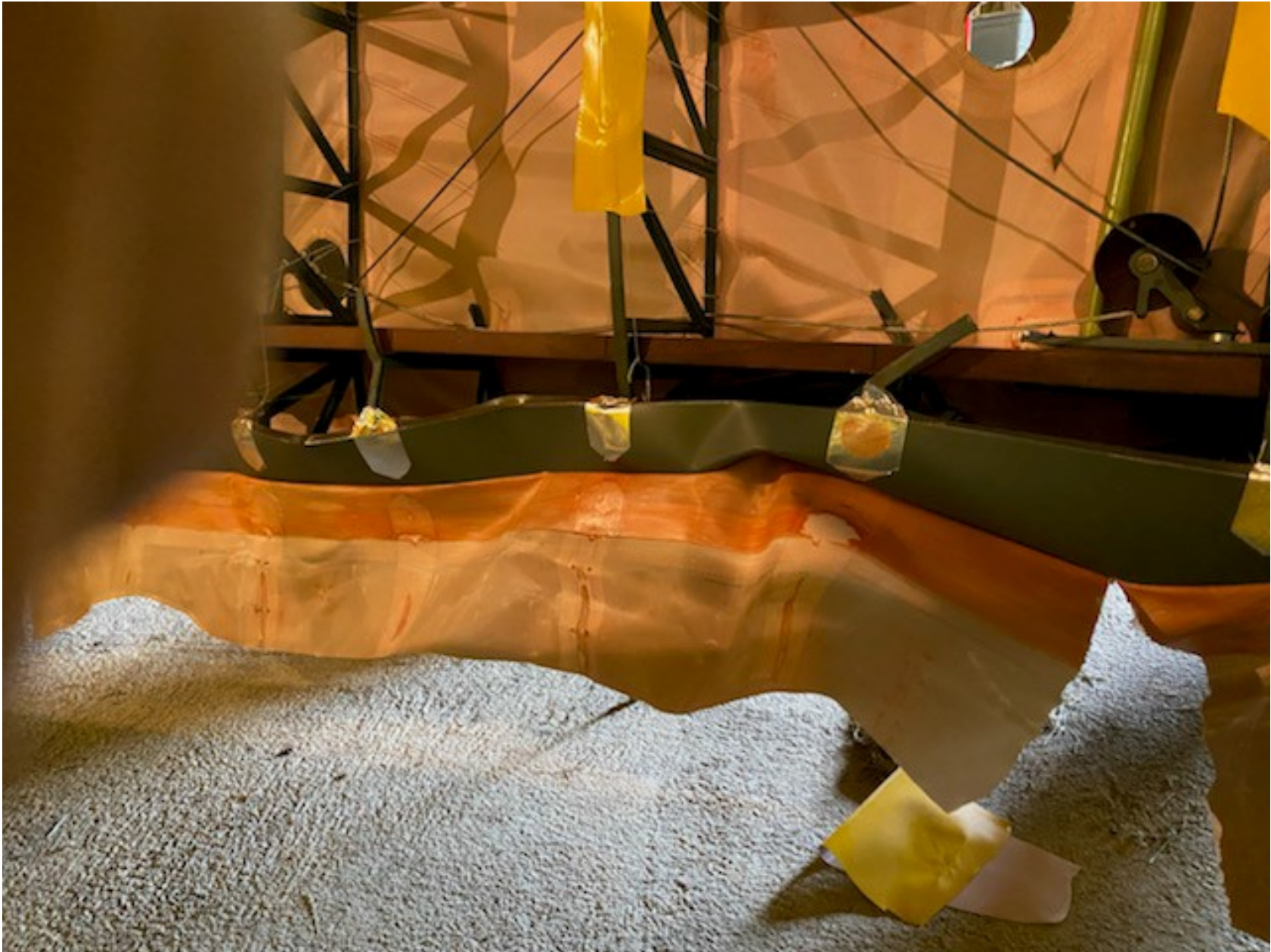
Photo 6 – No damage to left wing main spar, but leading edge is bent and crushed, breaking one rib and buckling another (FAA photo)
