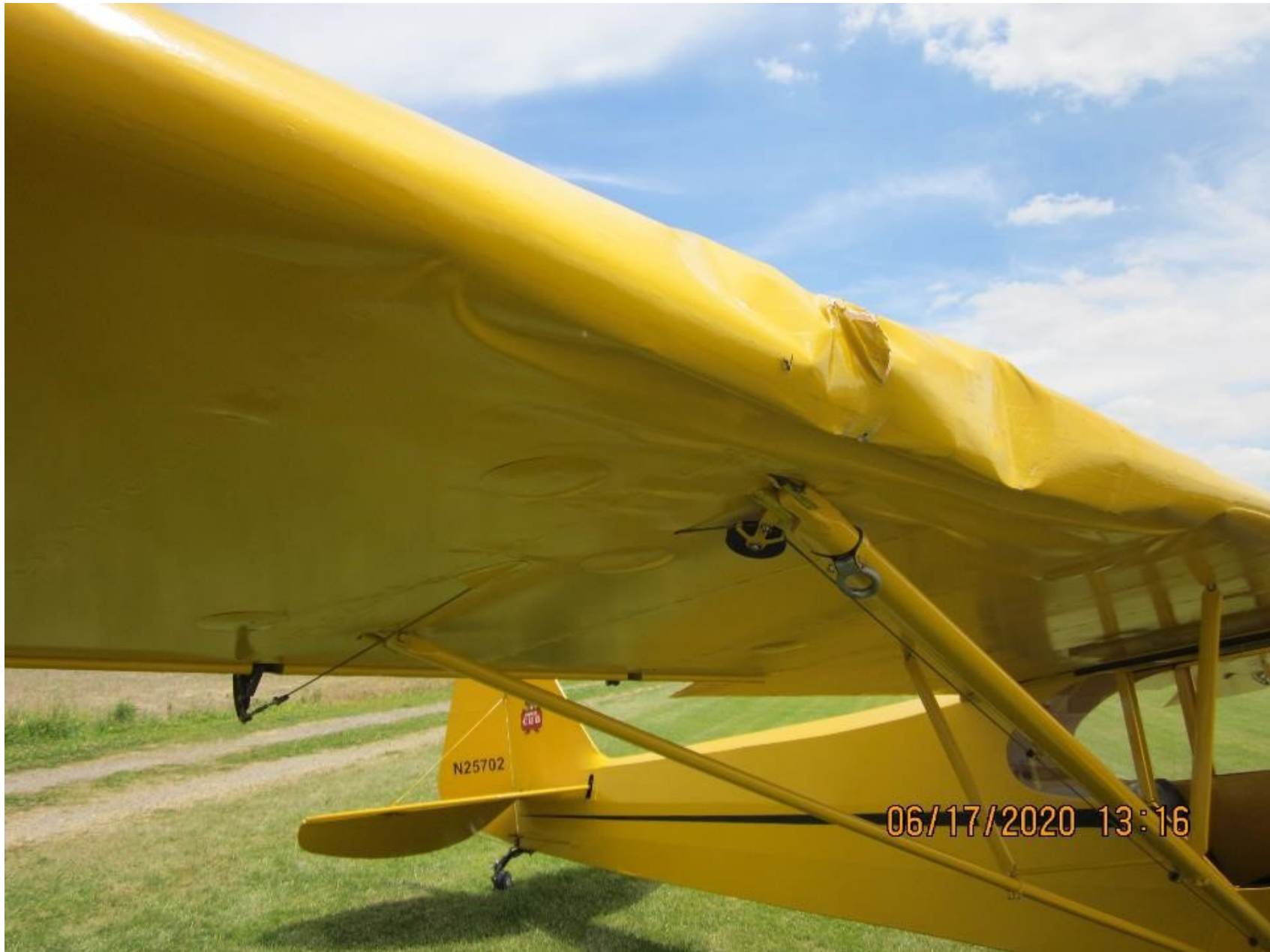
Photo 3 – Right wing leading edge damage (FAA photo)
