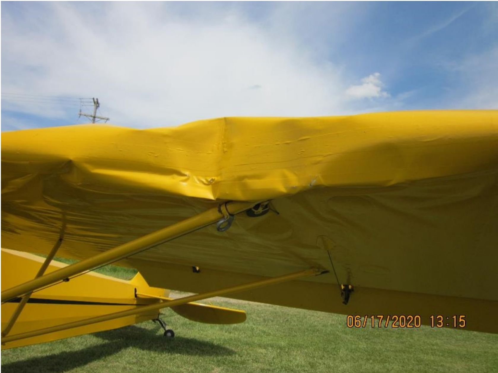
Photo 1 – Left wing leading edge damage (FAA photo)
