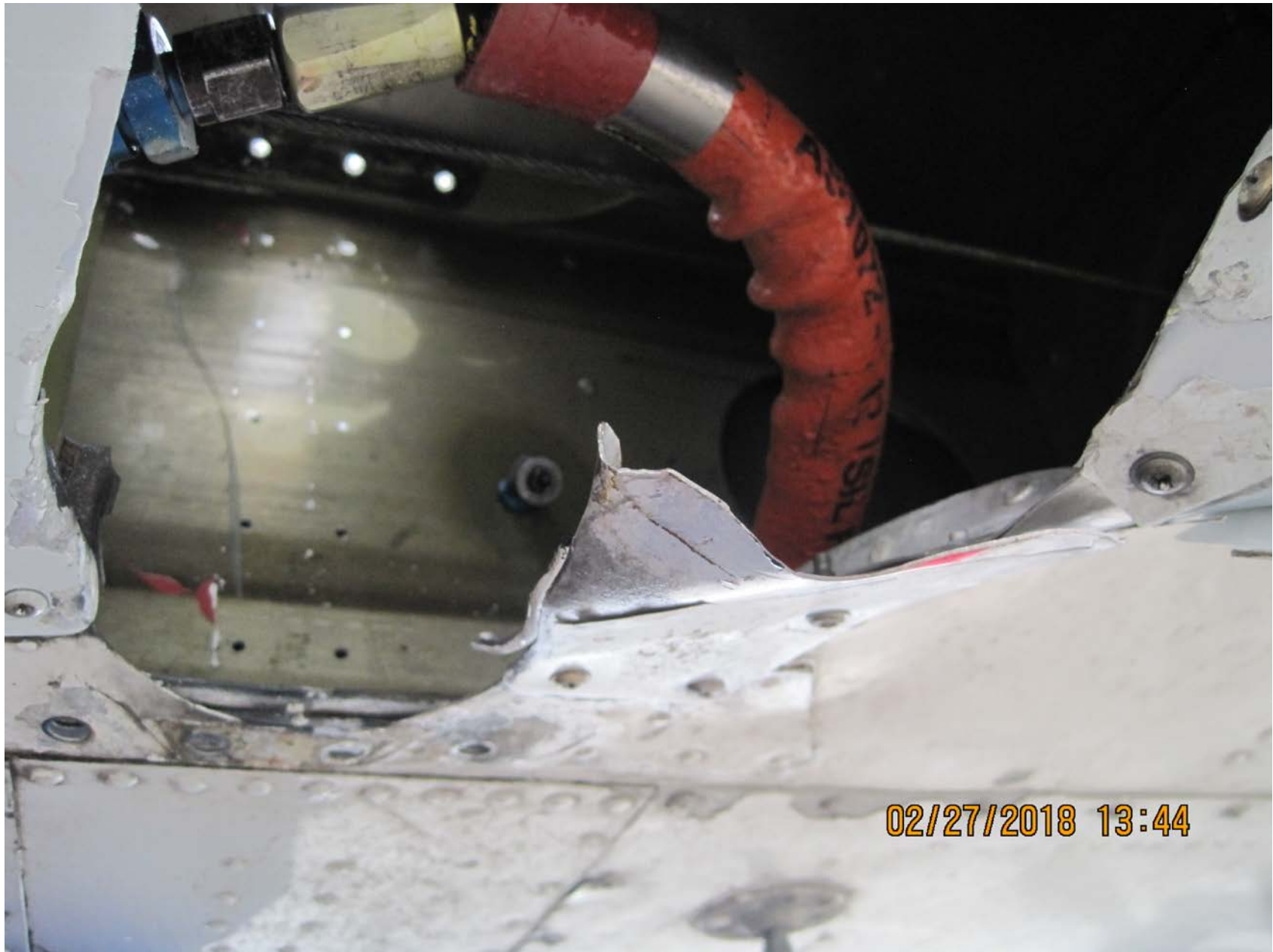
Photograph 3 – Lower right wing skin (provided by FAA)
