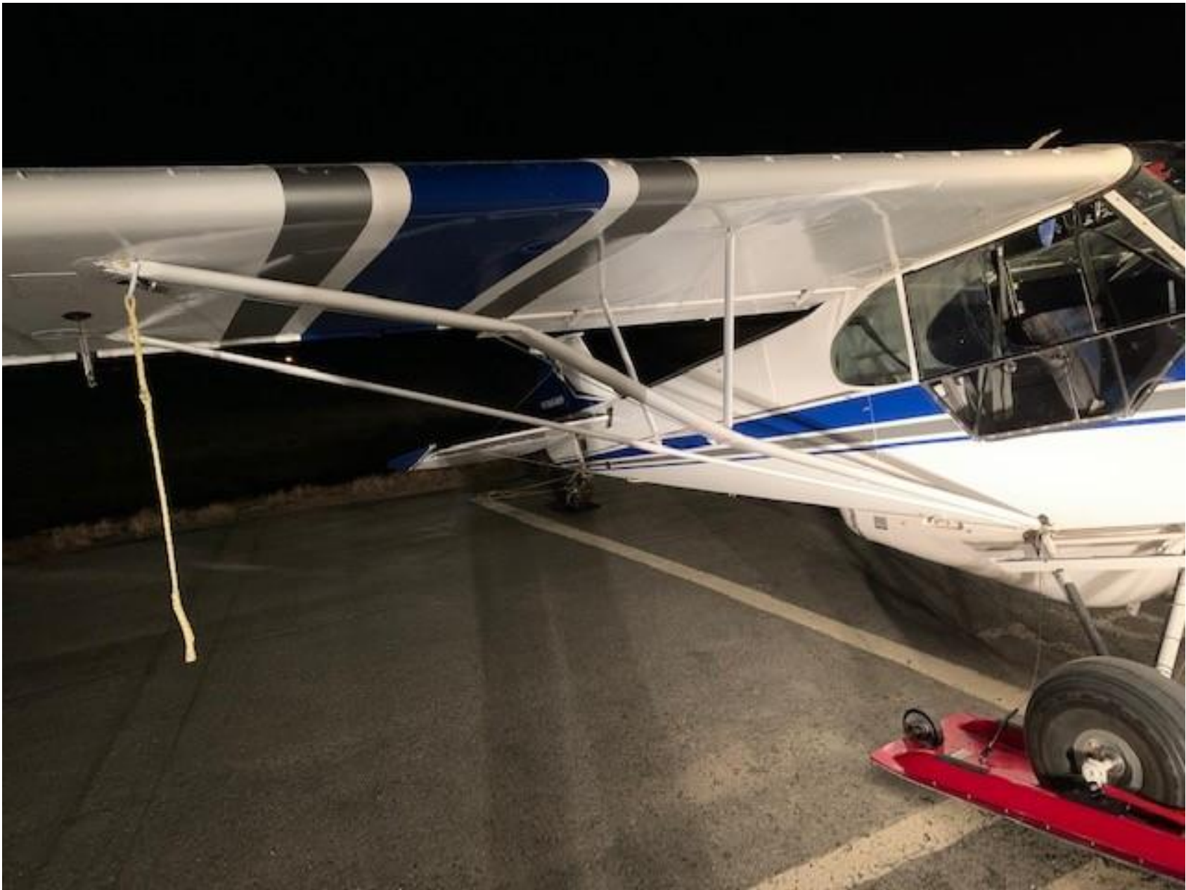
Photo 2 – View of damaged right wing lift strut (Photo courtesy of the airport manager)
