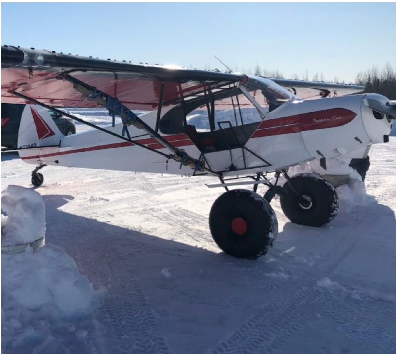
Photo 1 – View of damaged lift strut (Photo courtesy of the NTSB)
