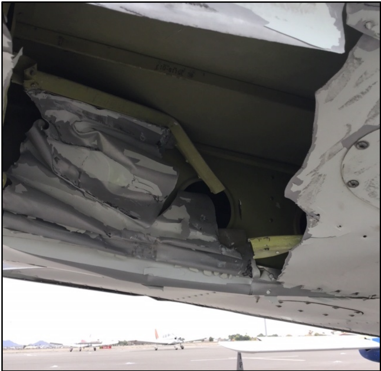
Image 1: Right wing damage as viewed from bottom.
