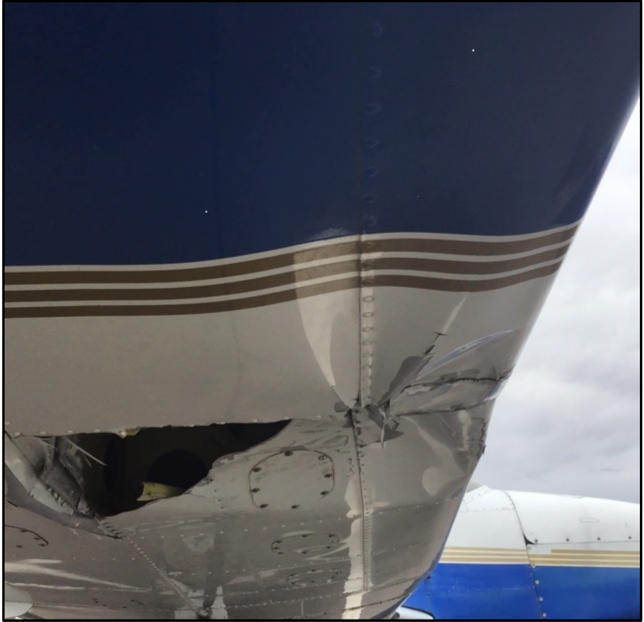
Image 2: Right wing damage as viewed from the right.
