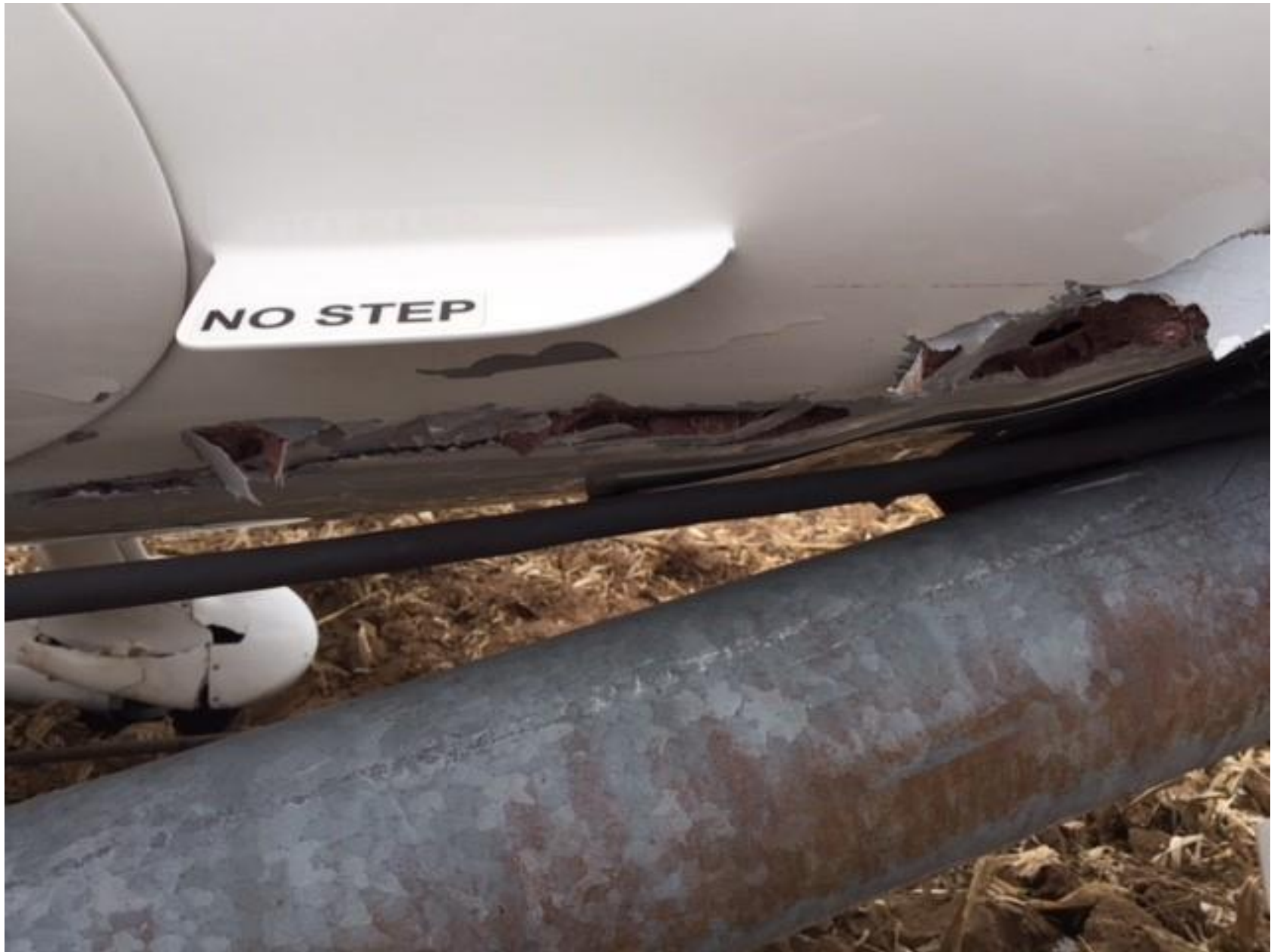
Photo 2 – View of damaged lower fuselage (Photo courtesy of the FAA)
