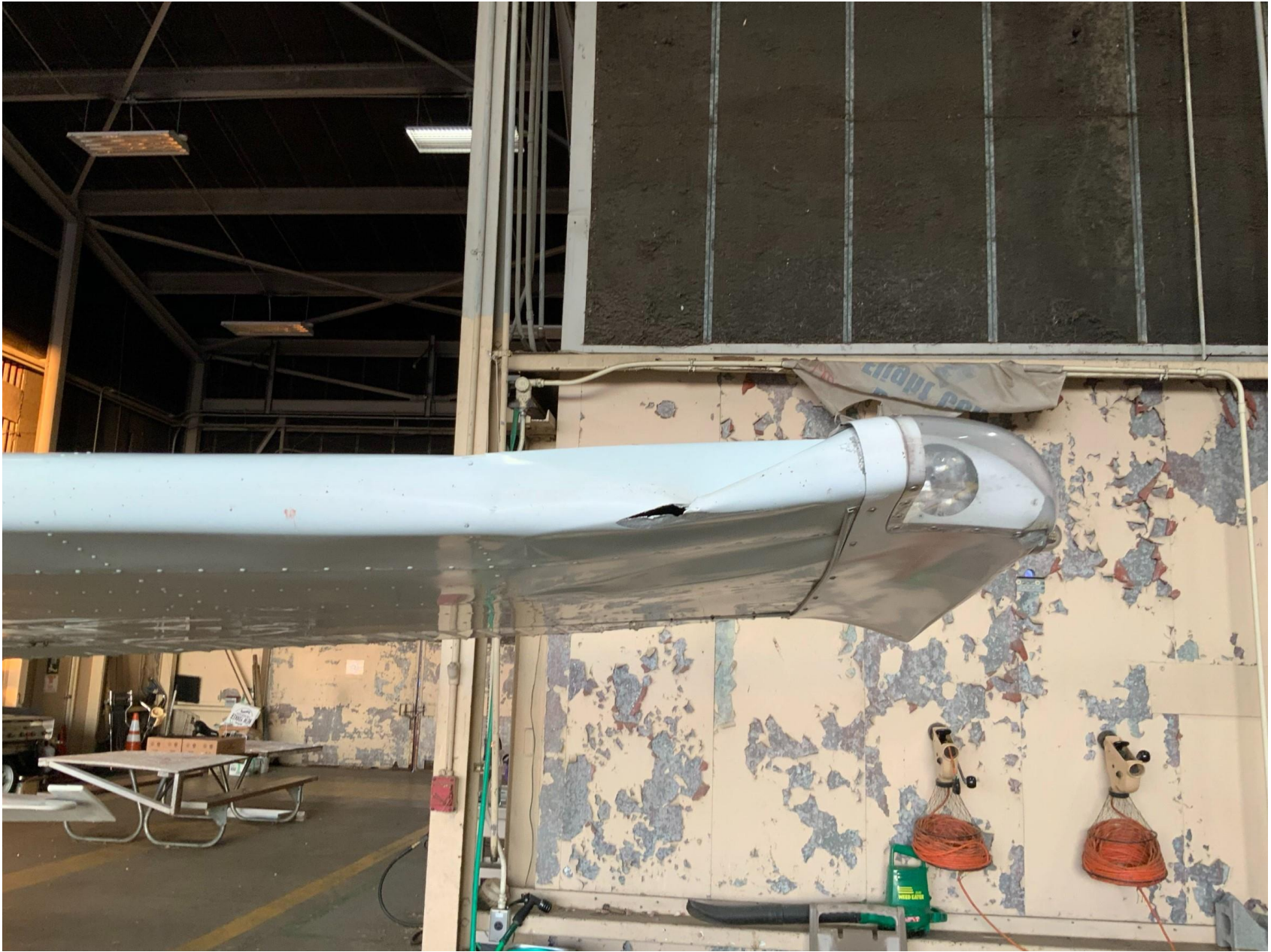
Photo 1 – View of damaged left wing (Photo courtesy of the Aero Club)
