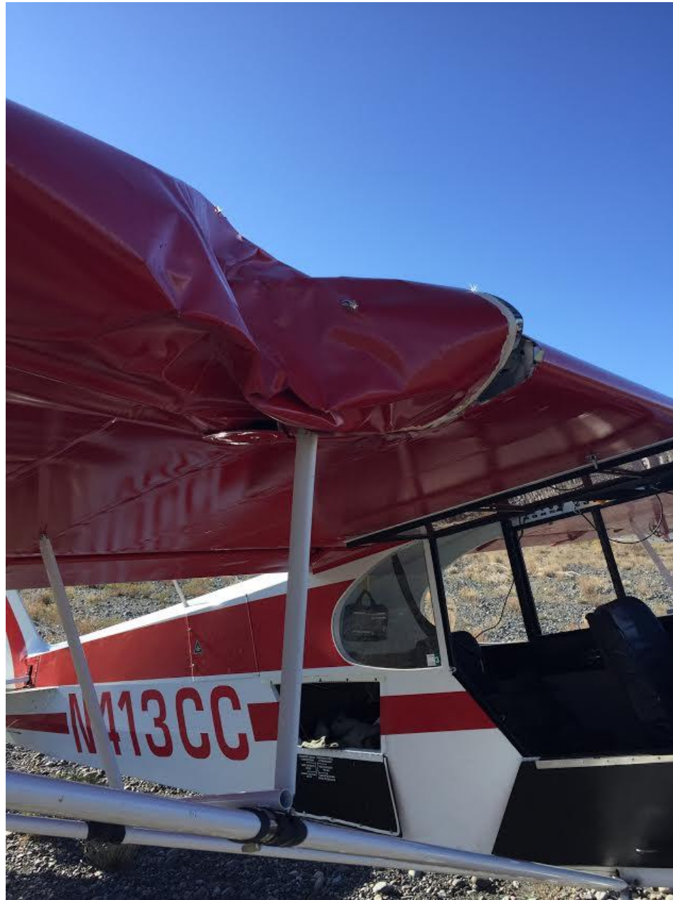
Photo 1 – View of damaged right wing (Photo courtesy of the Department of the Interior)
