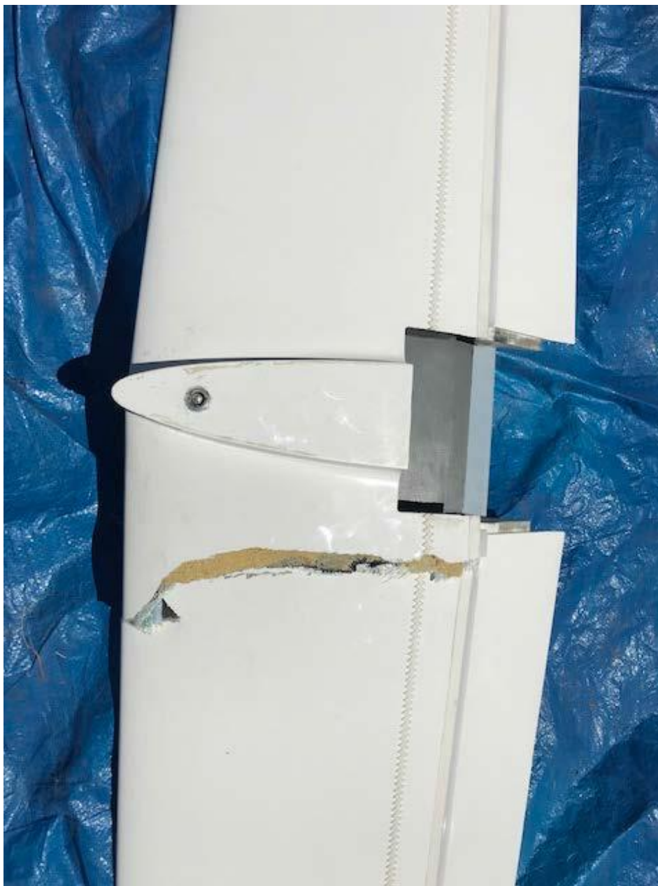
Photo 1 – View of damaged horizontal stabilizer (Photo courtesy of the FAA)
