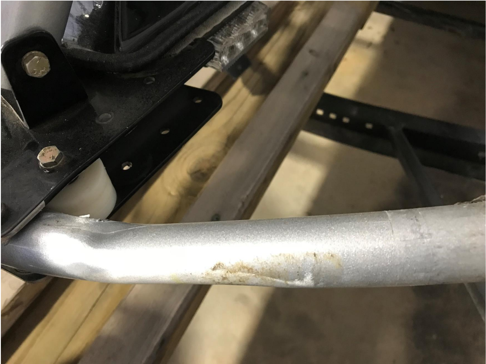
Photo 1 – View of left damaged steering bar (Photo courtesy of Pilot)
