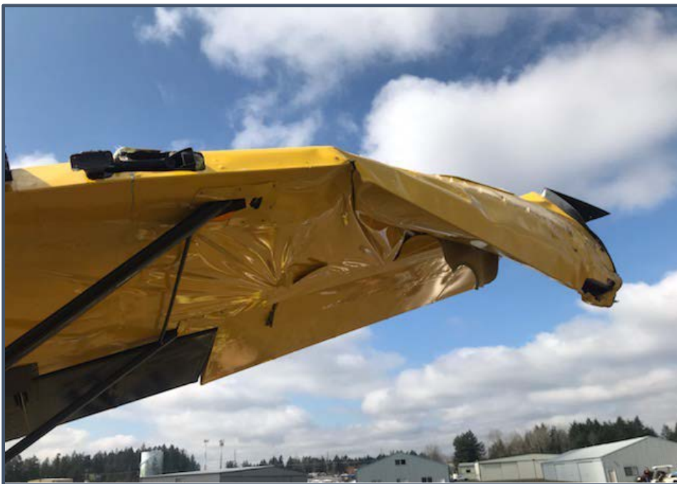
Figure 2: Airplane's damaged left wing (forward view).
