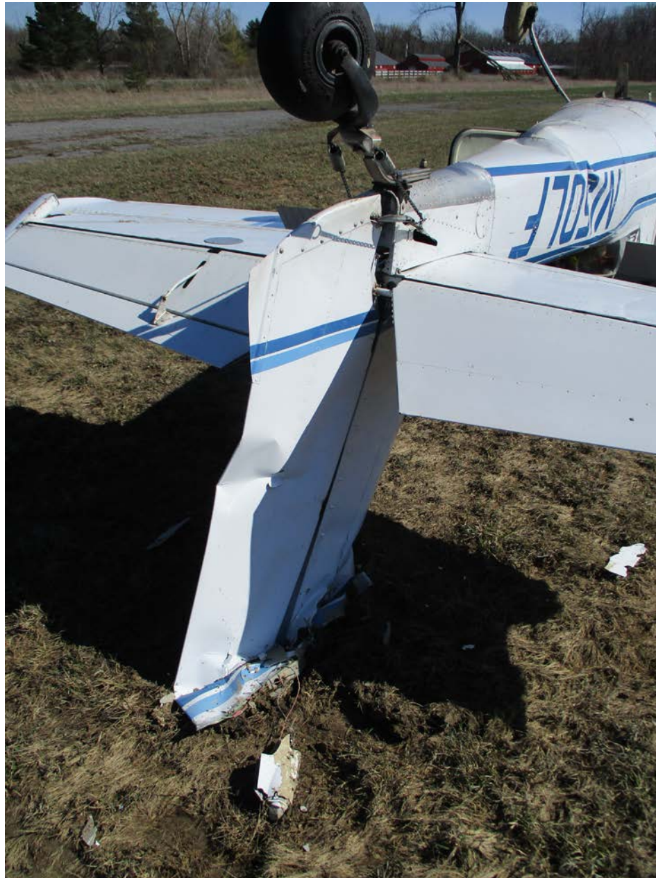
Photo 3 - View of vertical stabilizer and rudder damage (photo courtesy of the FAA)
