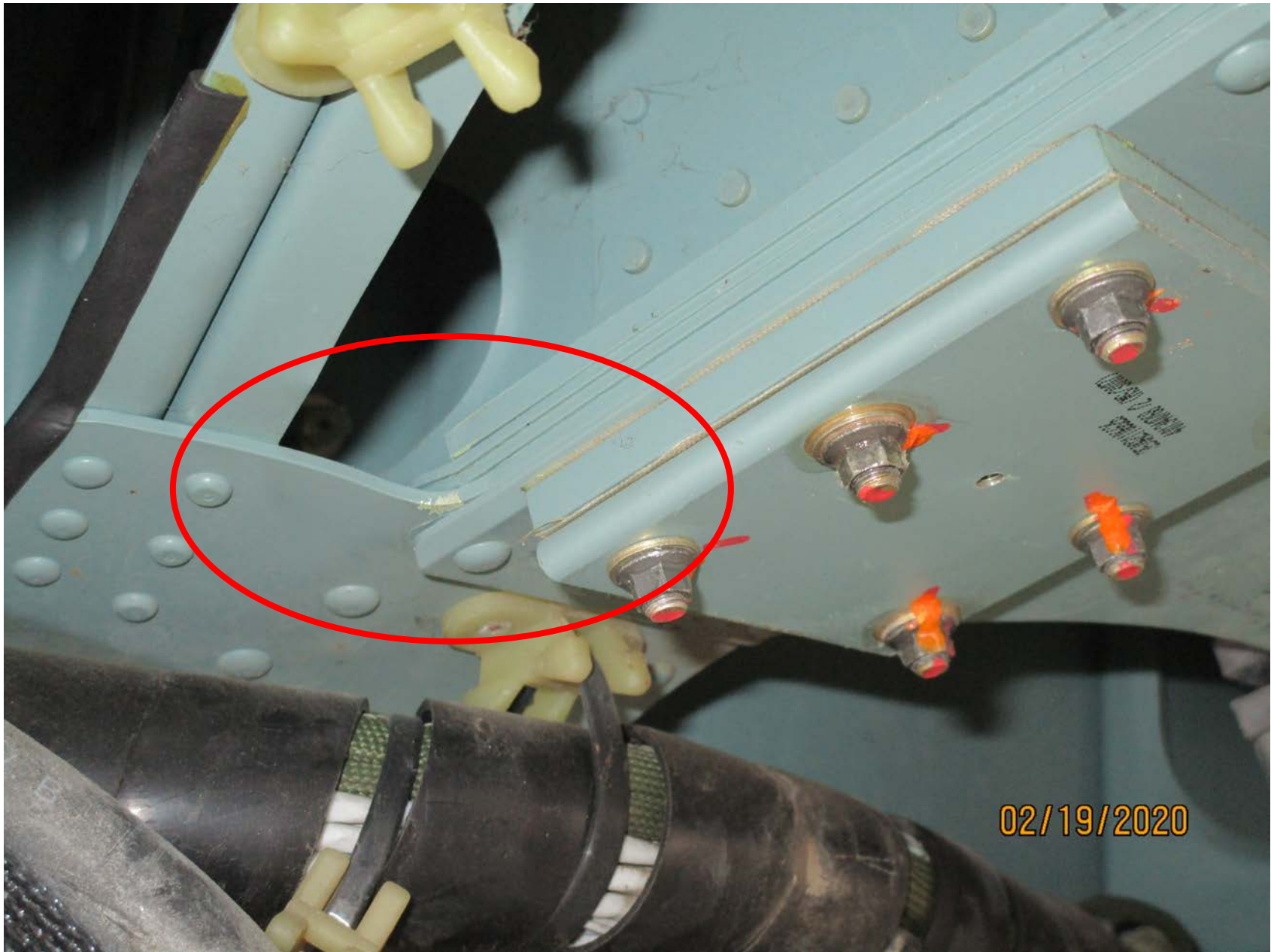
Photo 2 - View of left-hand anti-vibrator mount beam damage (photo courtesy of the FAA)
