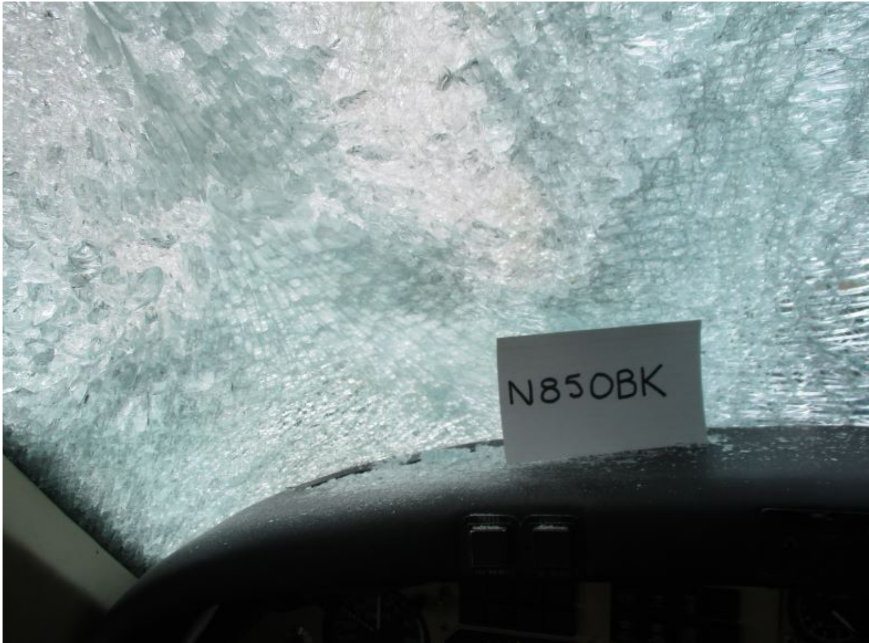
Photo 2 – View of damaged windshield from the pilot’s seat (courtesy of the FAA)
