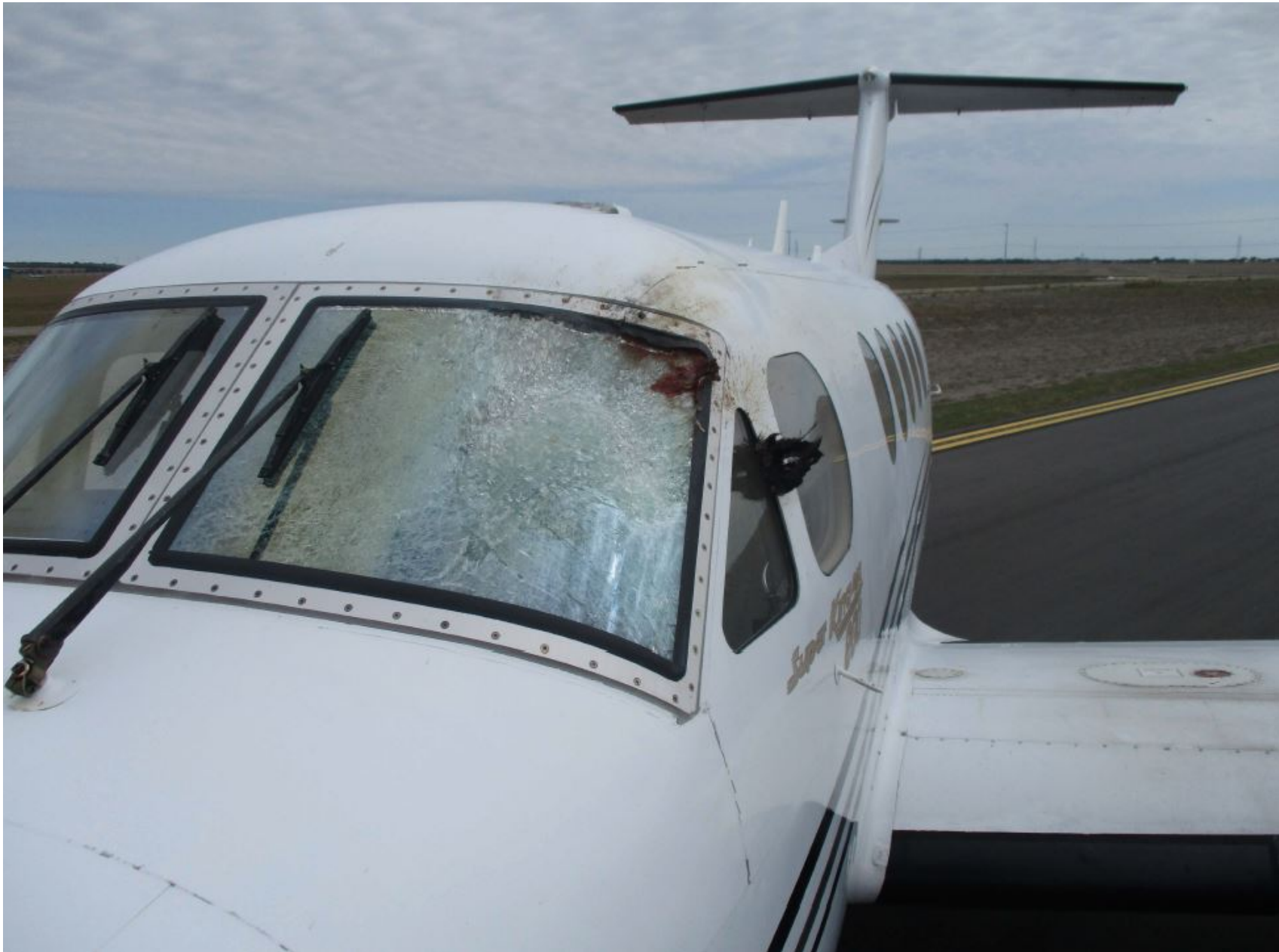
Photo 1 – View of damaged windshield from bird strike (courtesy of the FAA)
