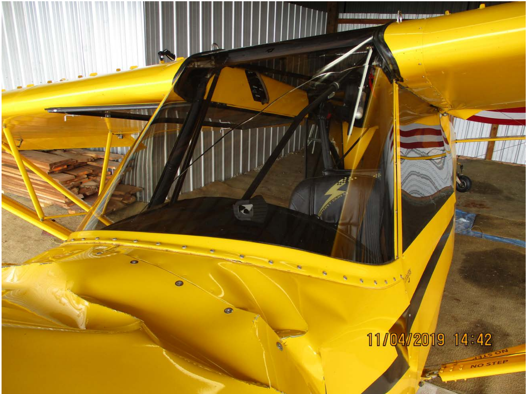
Photo 3 – View of damaged fuselage (courtesy of the FAA)
