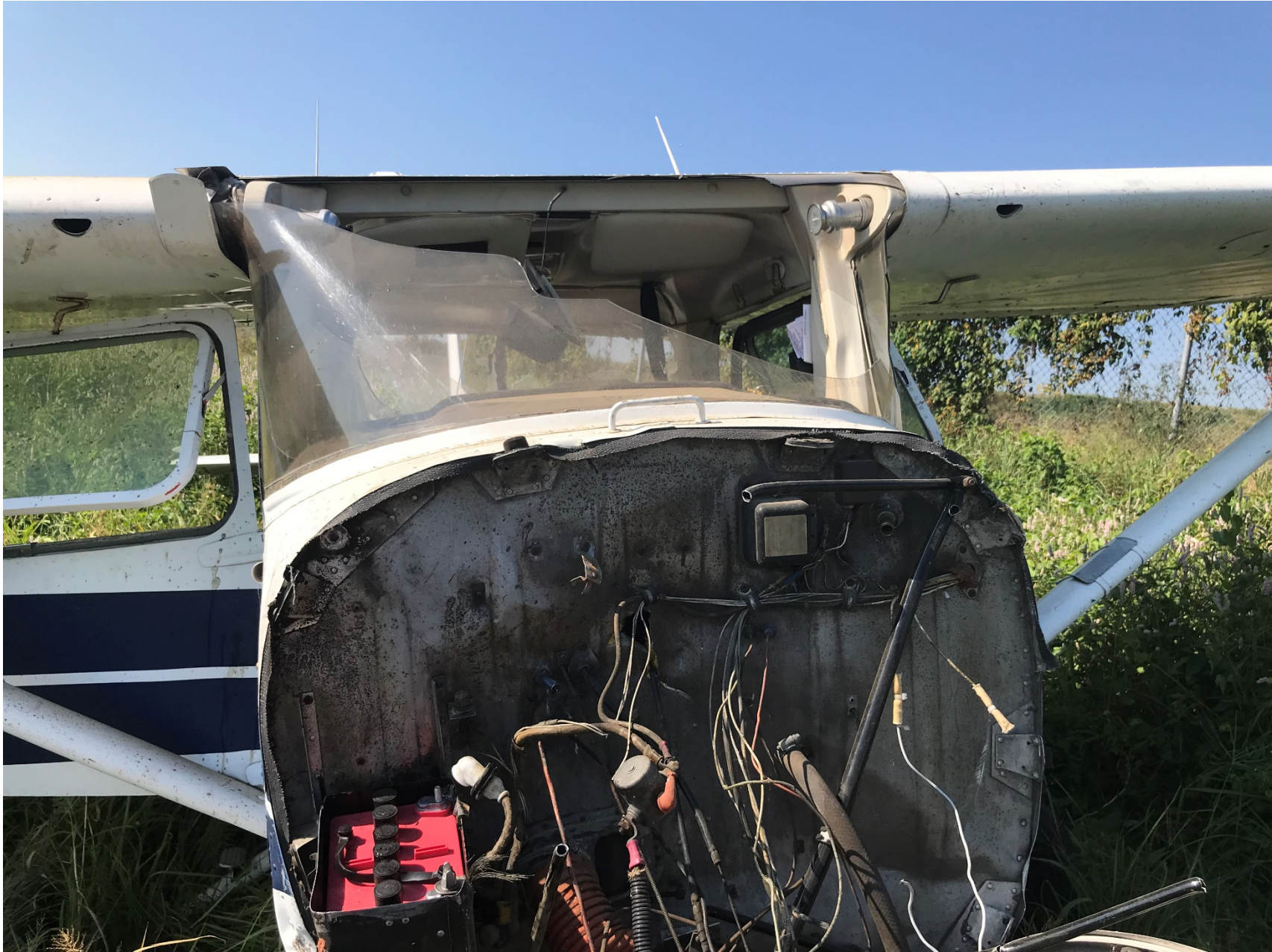
Photo 2 – View of damaged engine mounts (Photo courtesy of the FAA)
