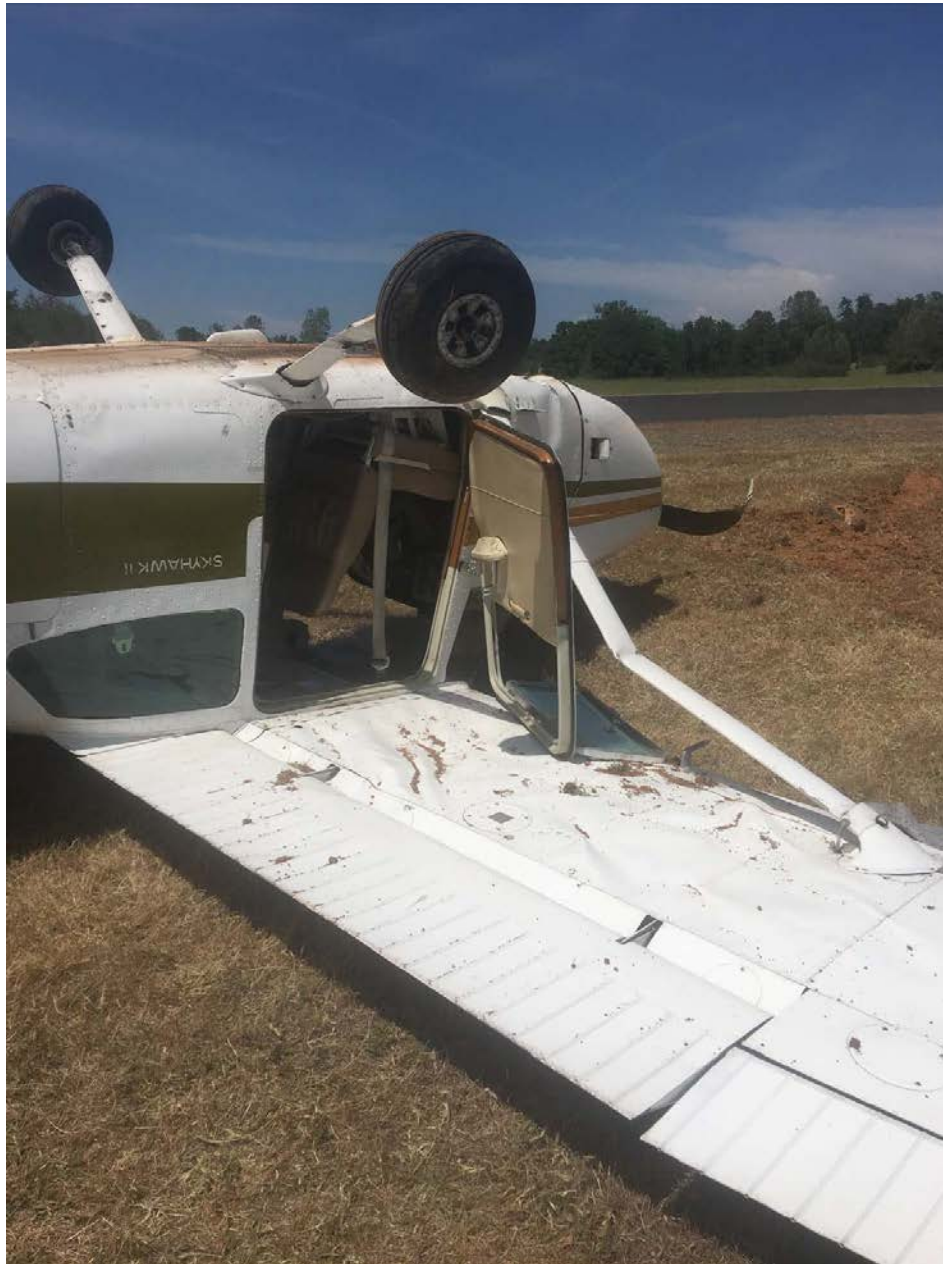
Photo 1 – View of damage to left-wing lift strut (courtesy of the FAA)
