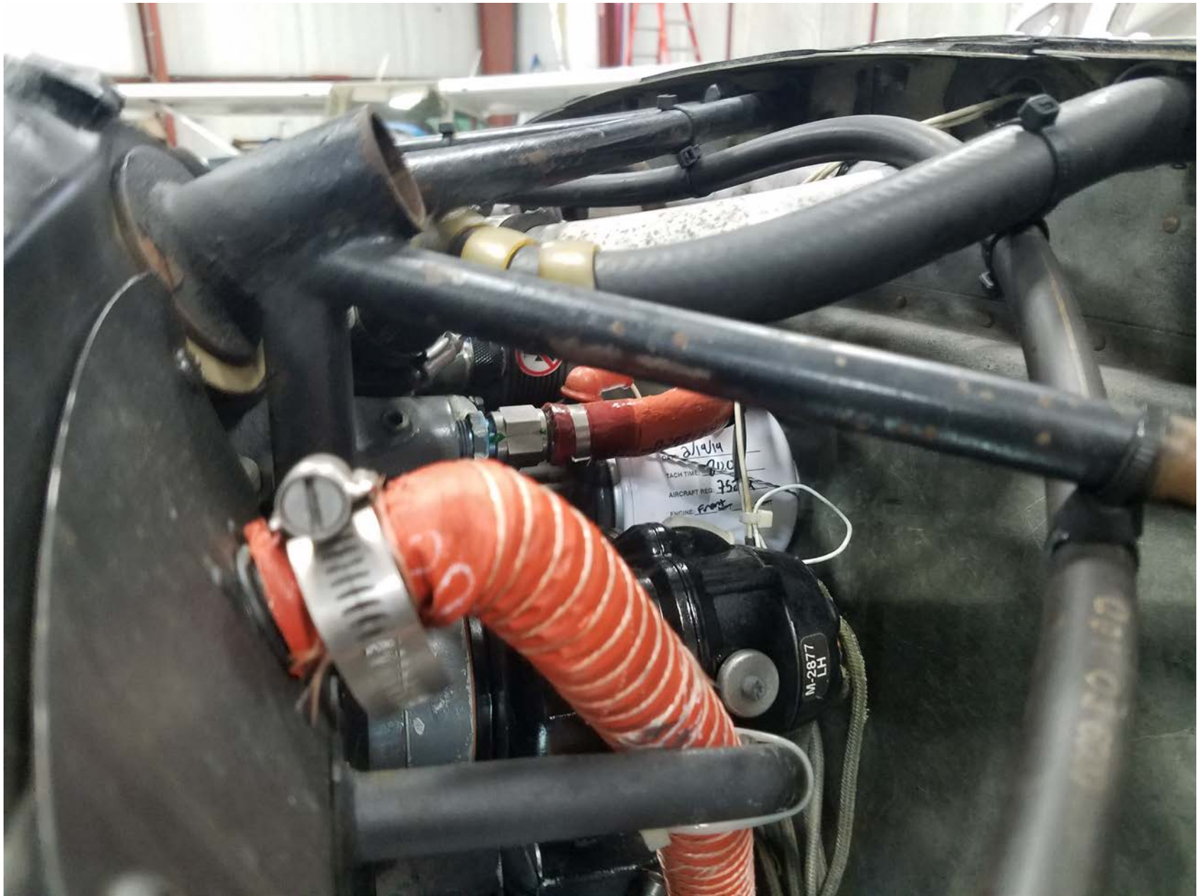
Photo 2 – View of damage to upper engine mount (courtesy of the FAA)
