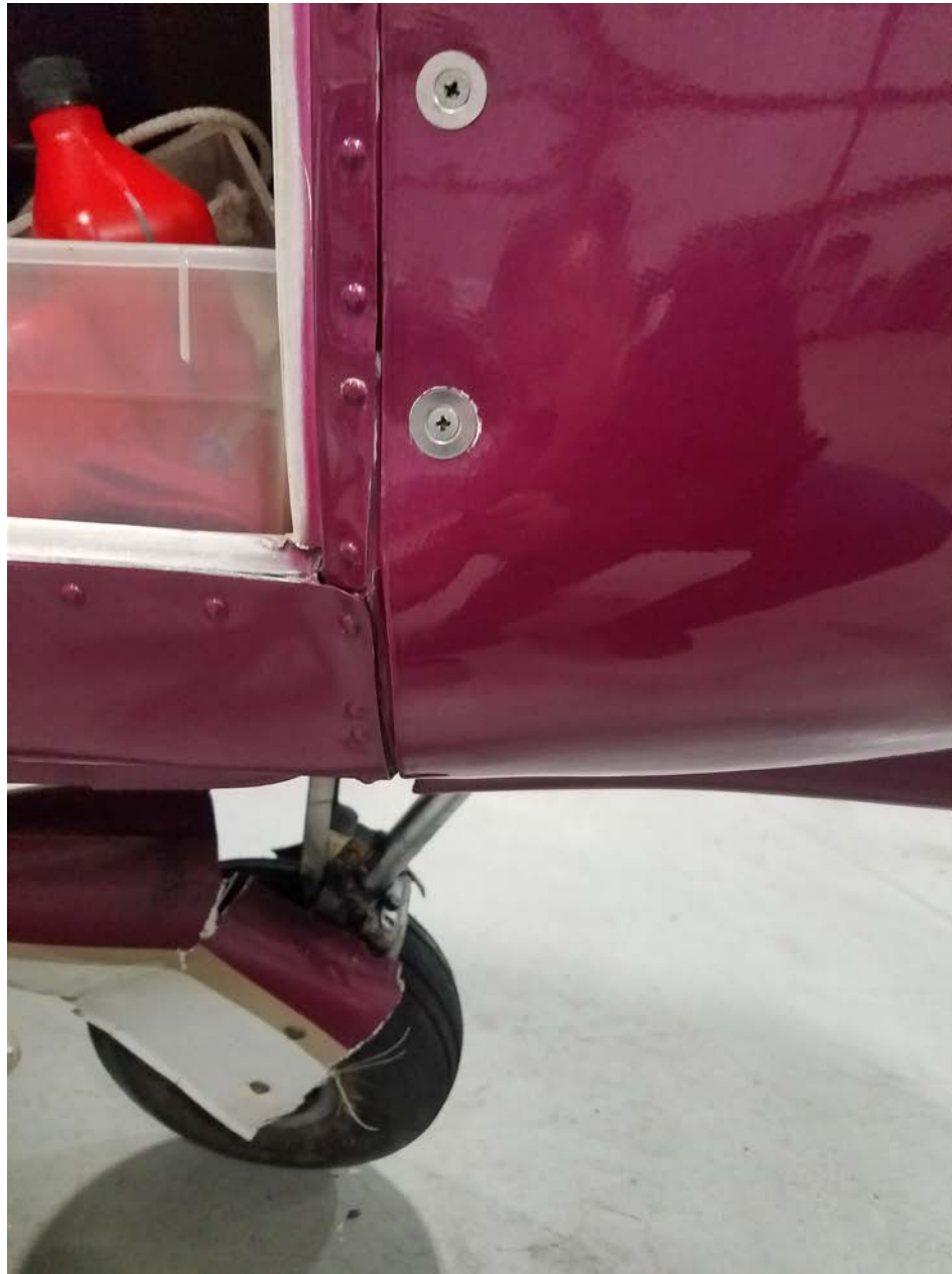
Photo 1 – View of damage to firewall (courtesy of the FAA)
