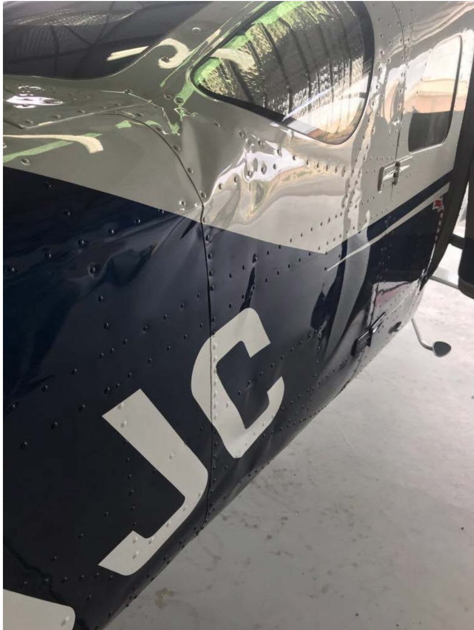
Photo 3 – View of fuselage damage on right side (Photo courtesy of the FAA)
