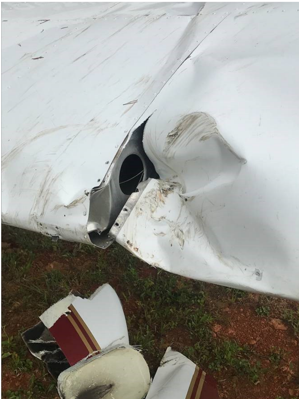
Photo 2 – View of left wing damage (Photo courtesy unknown)
