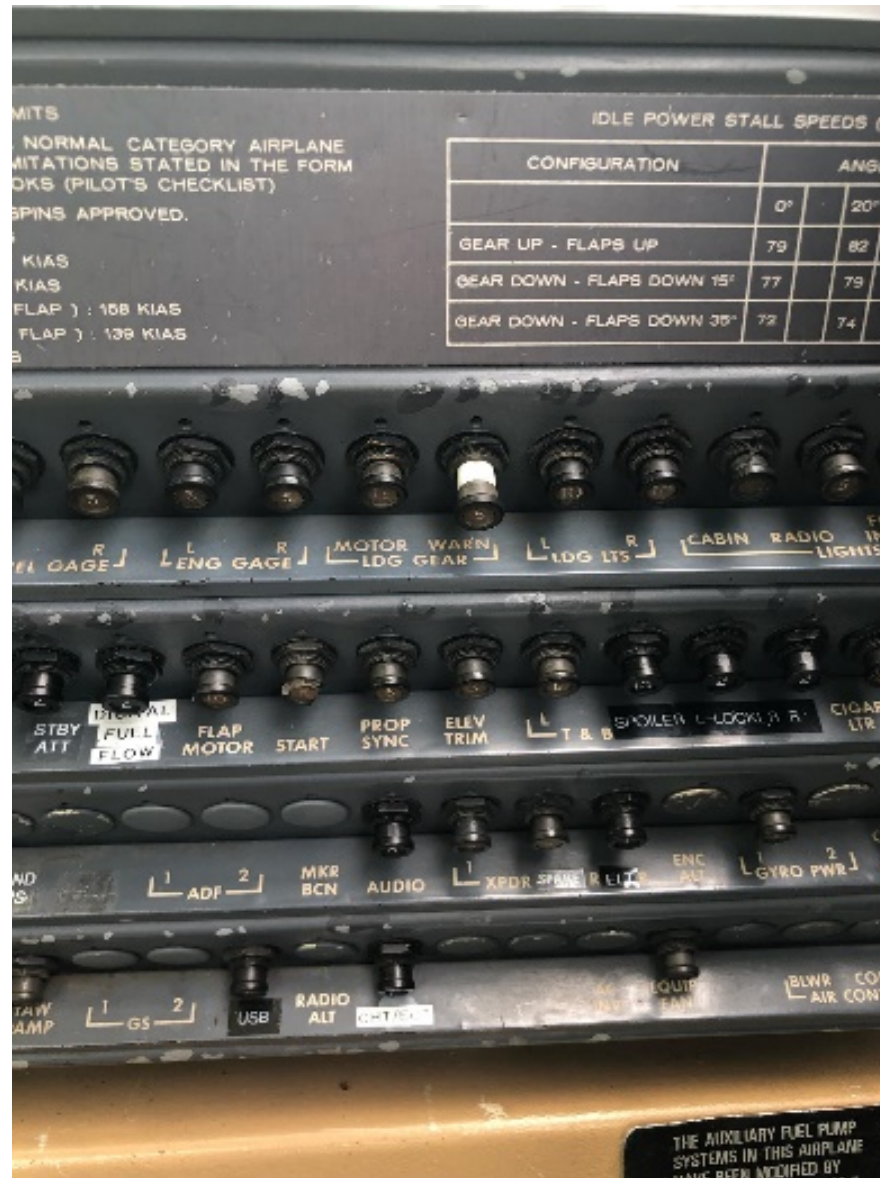
Photo 2 – View of example circuit breaker panel (Photo courtesy of the director of flight operations)
