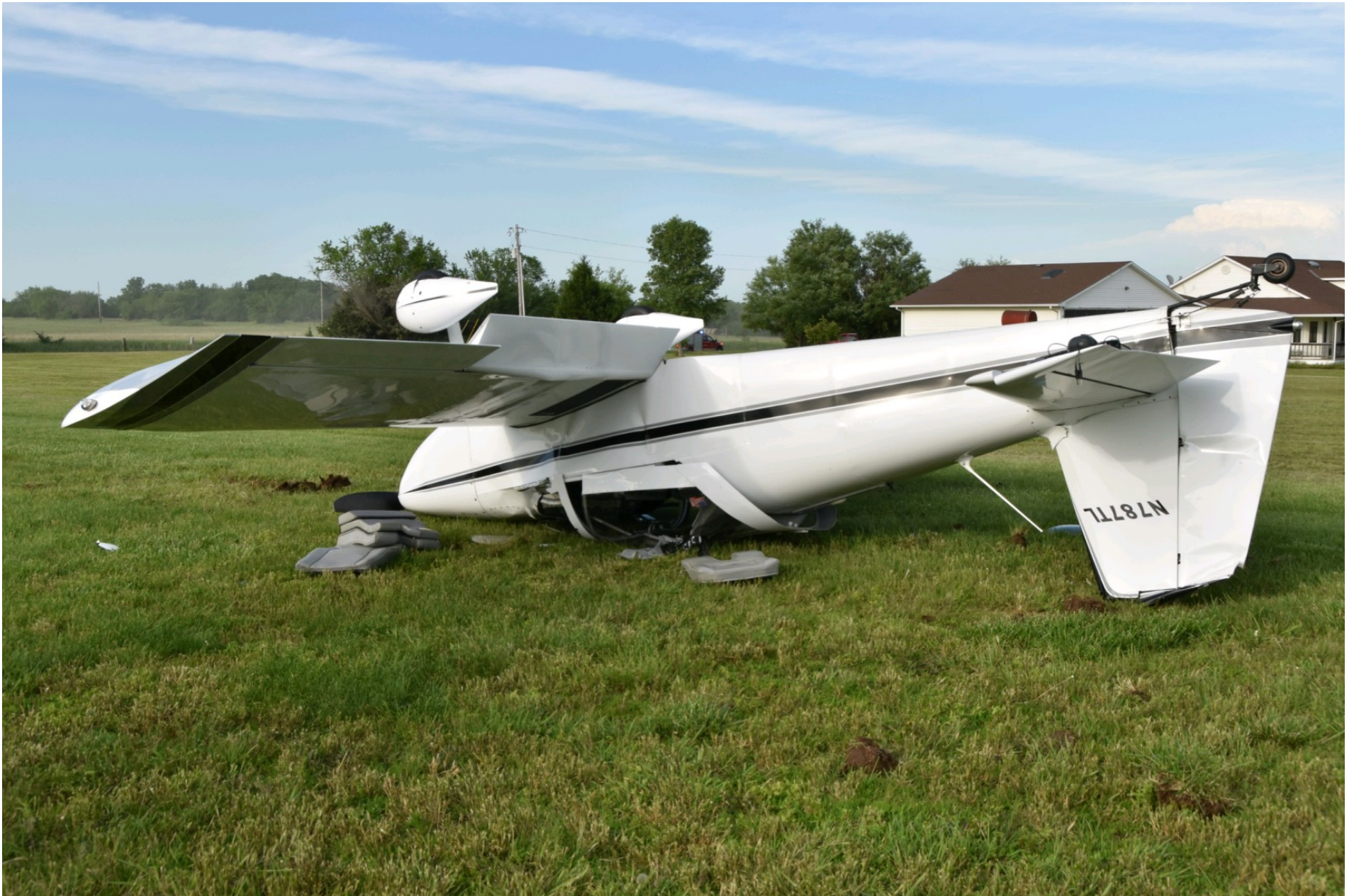
Photo 1 – View of fuselage and vertical stabilizer damage (photo courtesy of the pilot)
