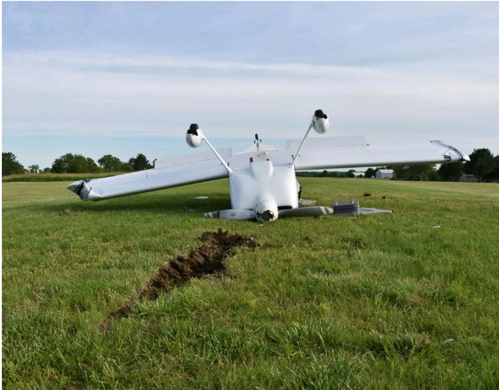
Photo 2 - View of damage to both wings (photo courtesy of the pilot)
