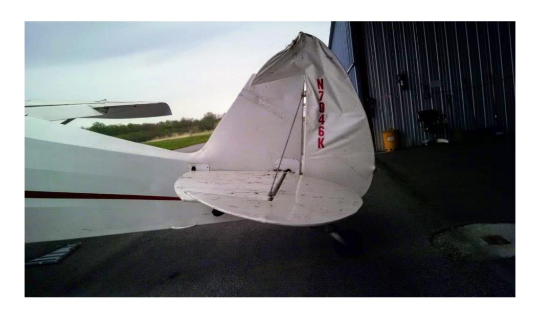
Photo 2 – View of damaged rudder (Photo courtesy of the insurance adjuster)
