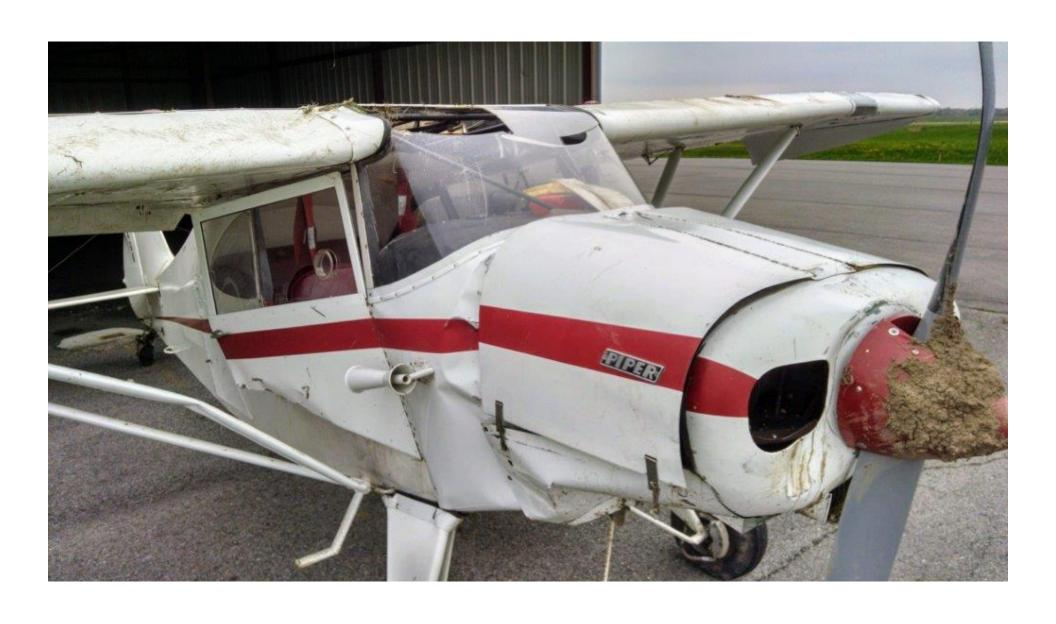
Photo 1 – View of damaged right wing lift strut and fuselage (Photo courtesy of insurance adjuster)
