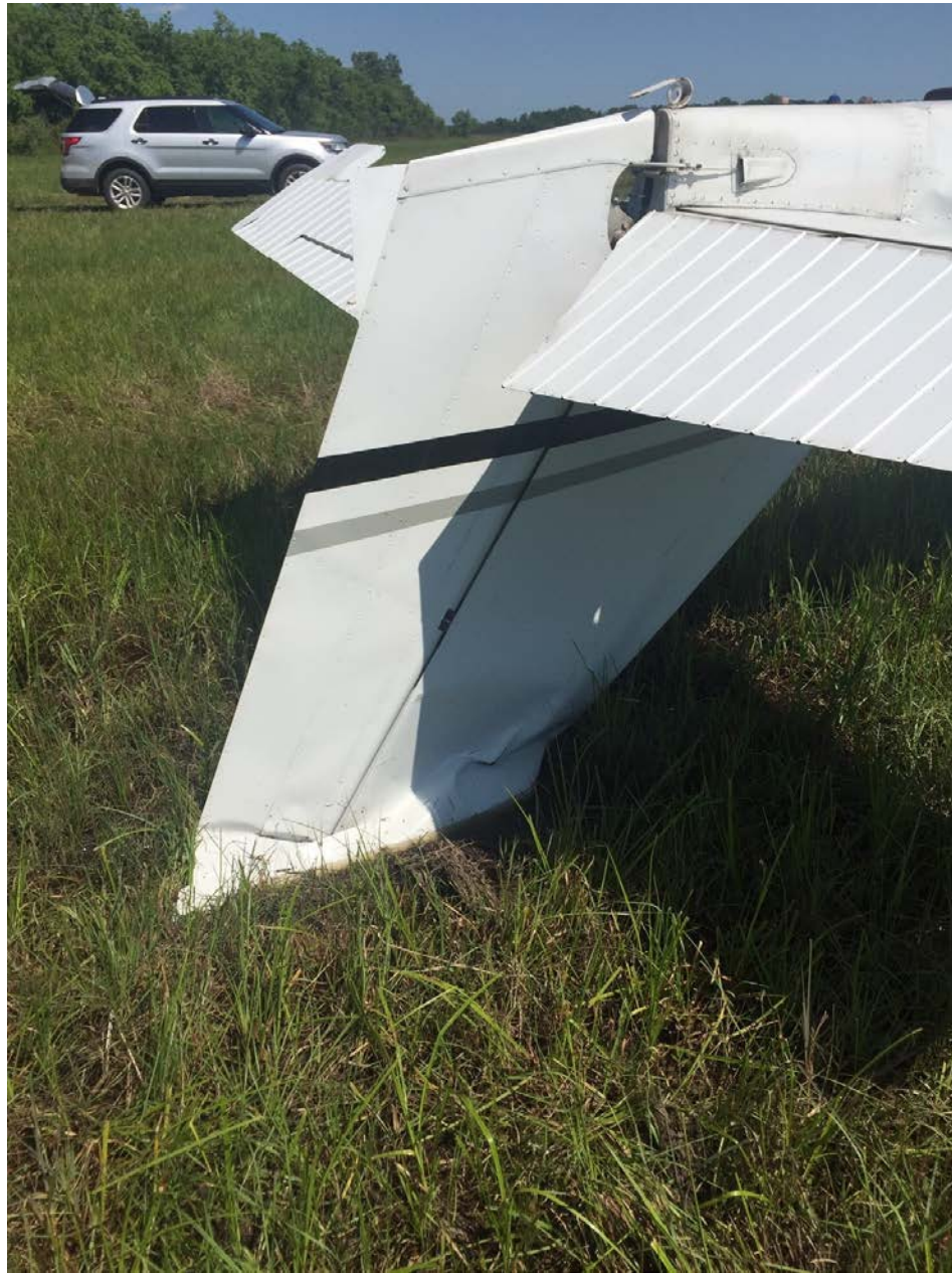
Photo 4 - View of vertical stabilizer damage (photo courtesy of the FAA)
