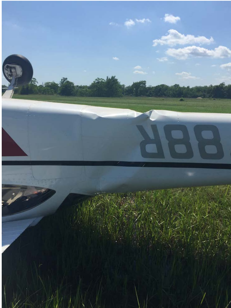
Photo 2 - View of aft fuselage damage (photo courtesy of the FAA)
