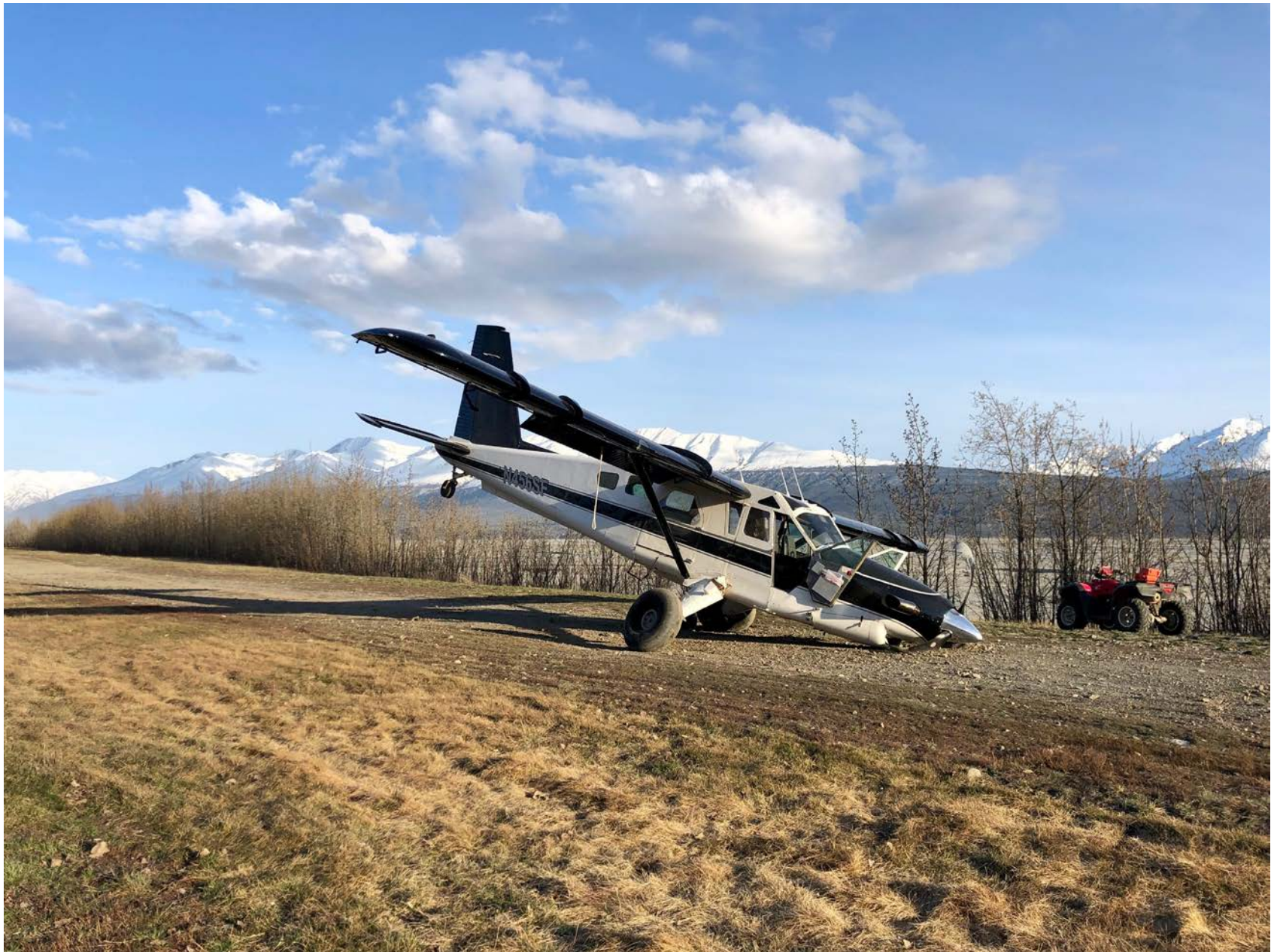
Photo 1 – View of right landing gear support damage (photo courtesy of the pilot)
