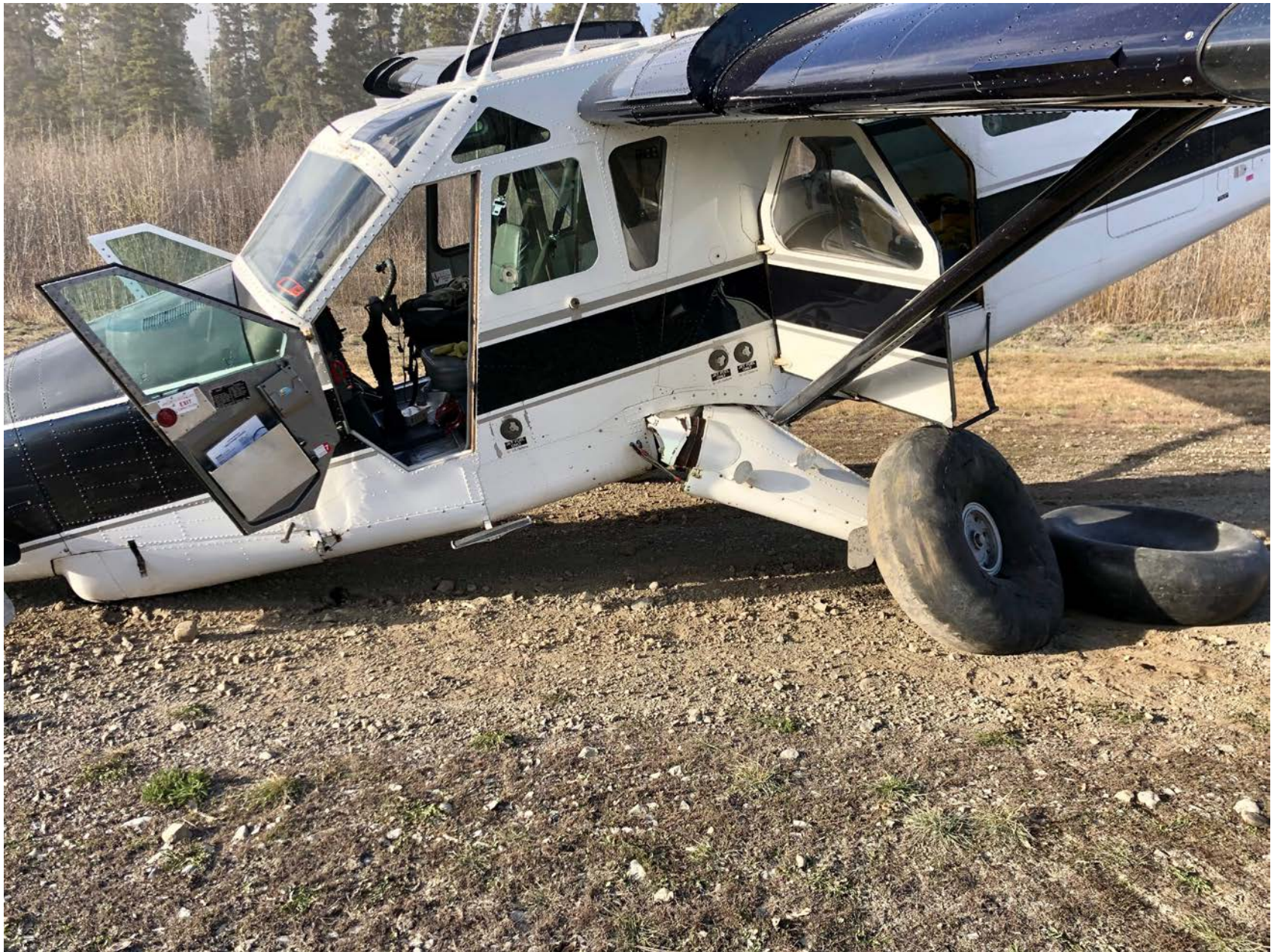
Photo 2 - View of left landing gear support damage (photo courtesy of the pilot)
