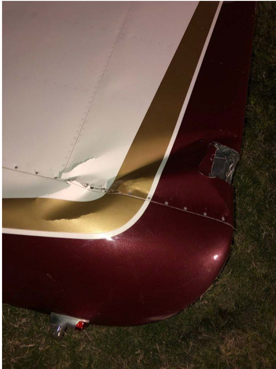
Photo 3 - View of left wing damage (photo courtesy of the FAA)
