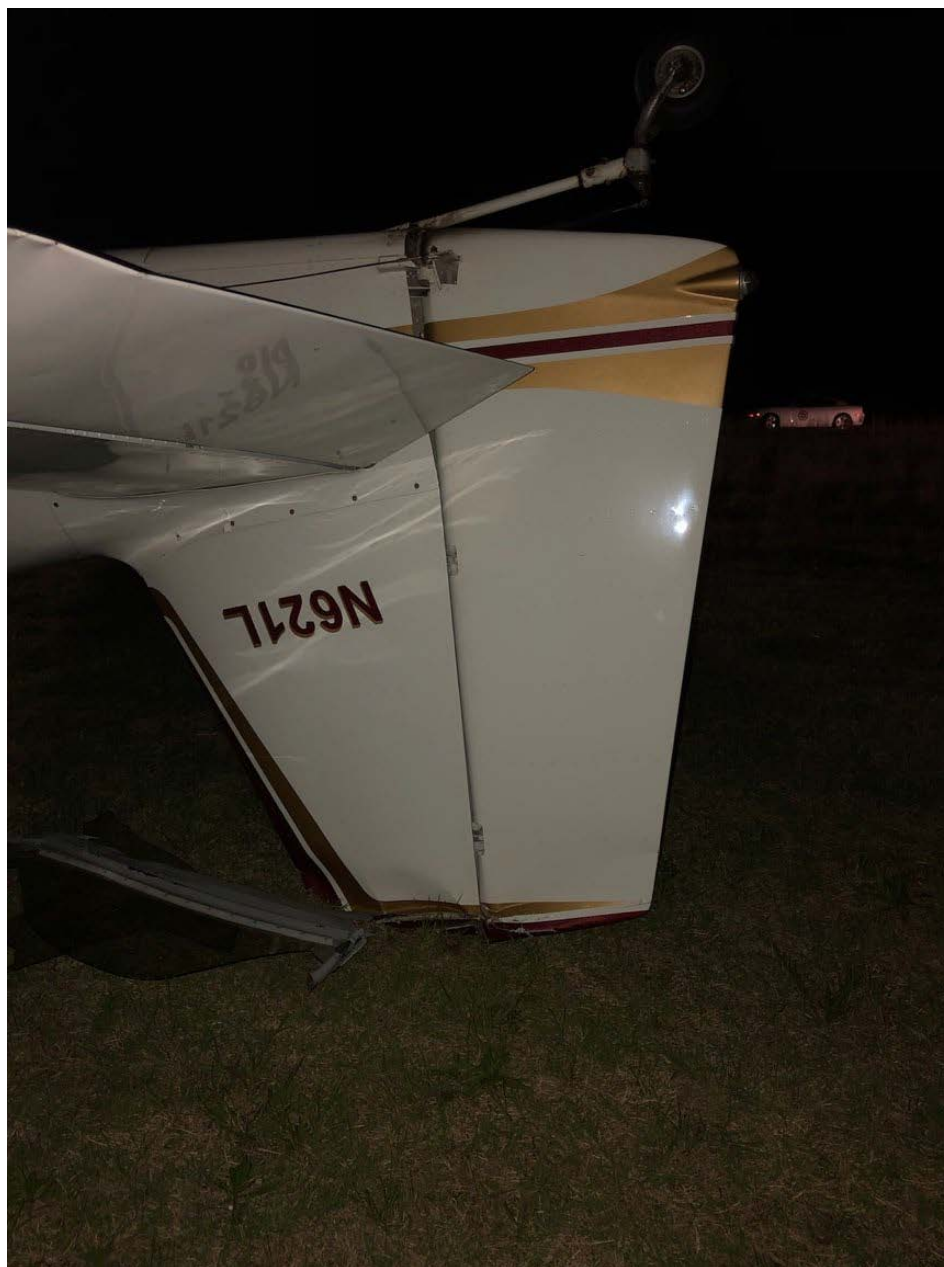
Photo 2 - View of vertical stabilizer damage (photo courtesy of the FAA)
