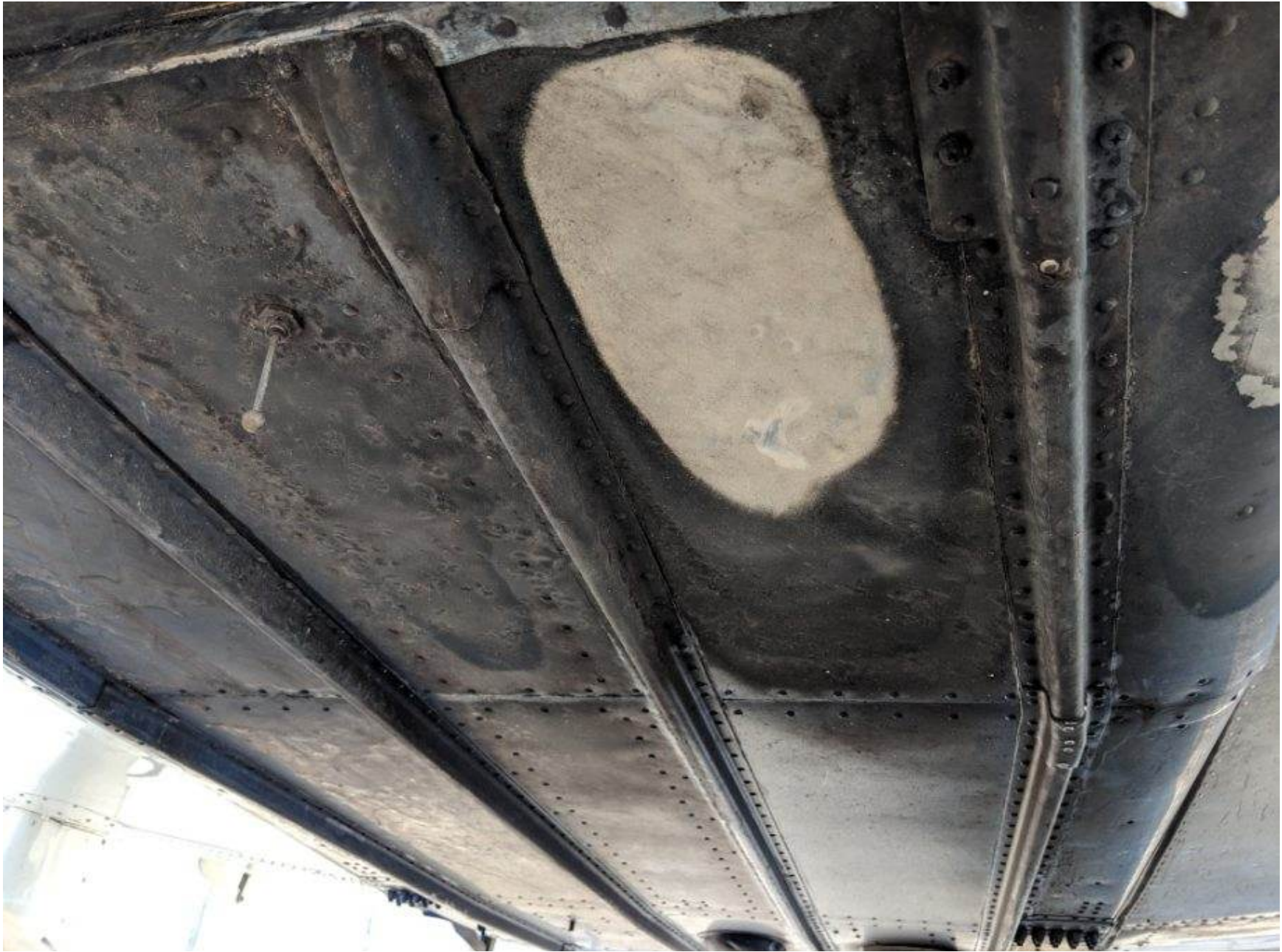
Photo 2 – View of damaged fuselage from below (Photo courtesy of the FAA)
