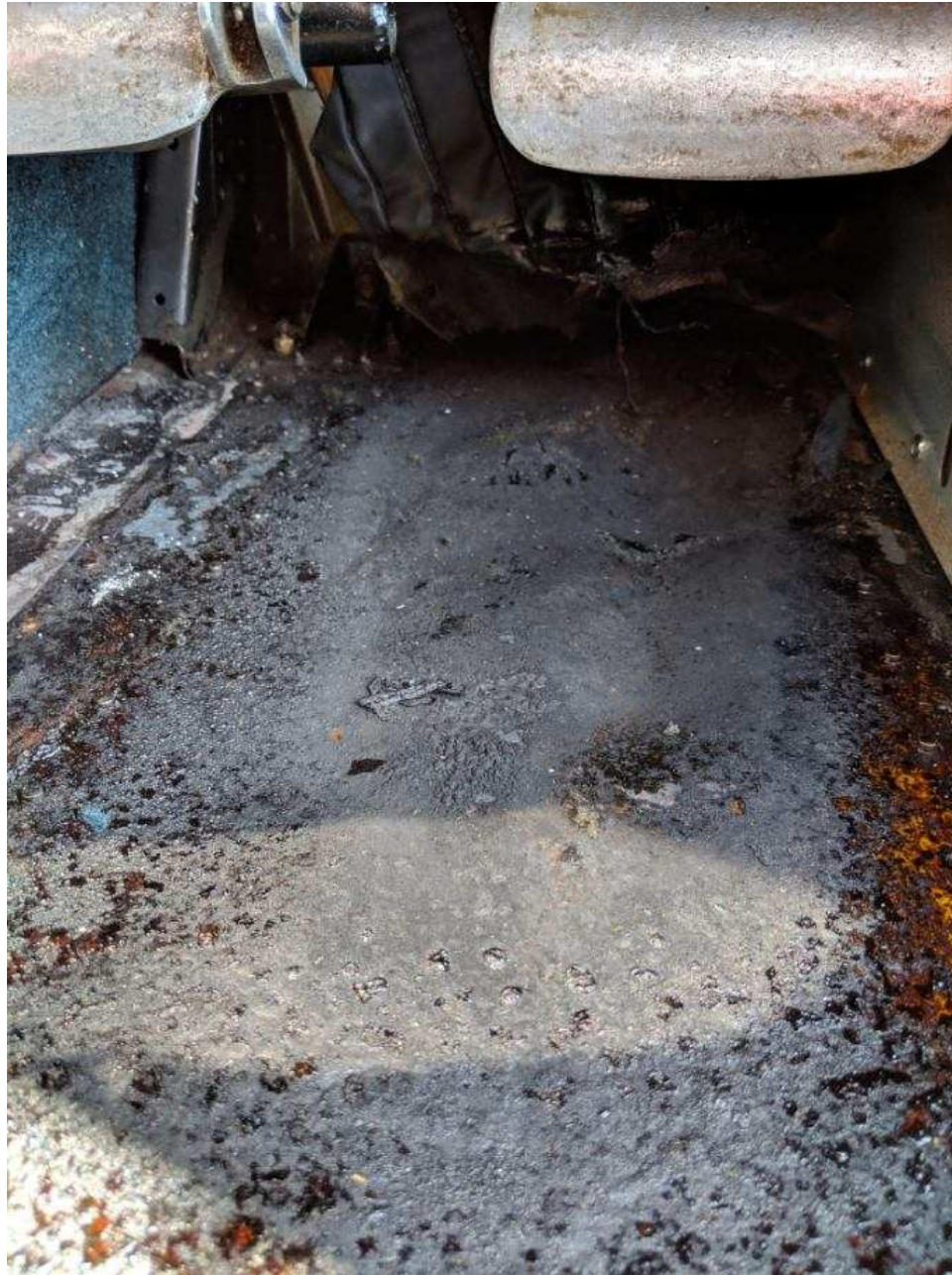
Photo 3 – View of damaged pilot side floorboards (Photo courtesy of the FAA)
