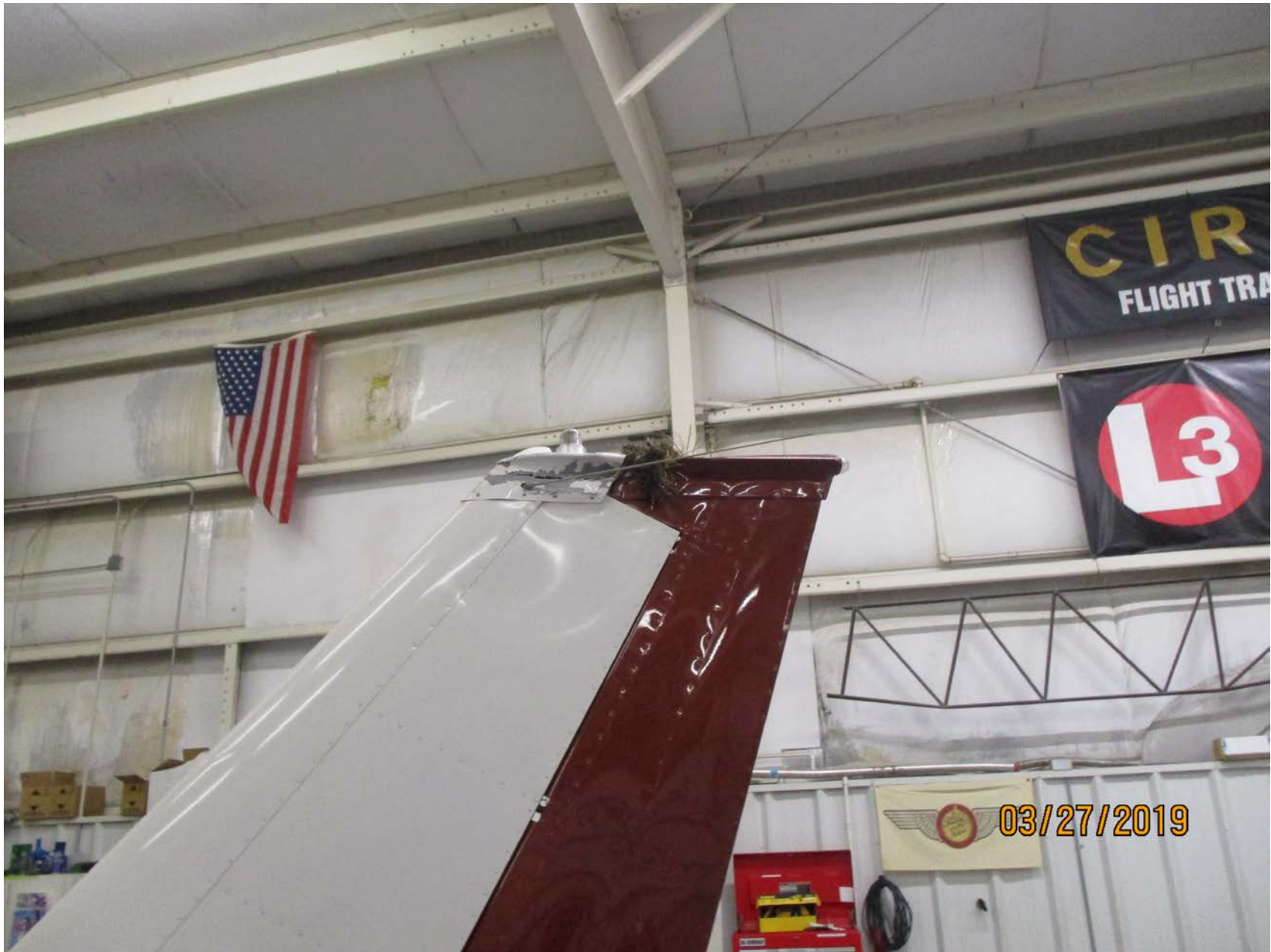
Photo 2 - View of rudder damage (photo courtesy of the FAA)
