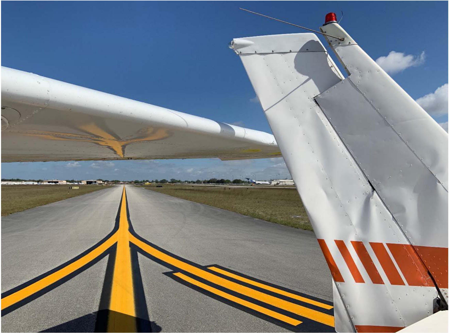
Photo 1 – View of damaged vertical stabilizer and rudder of N704VM (Photo courtesy of the airport operations)
