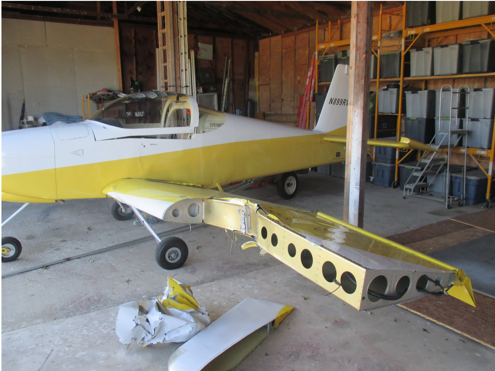
Photo 2 – View of damaged left wing spar (Photo courtesy of the FAA)
