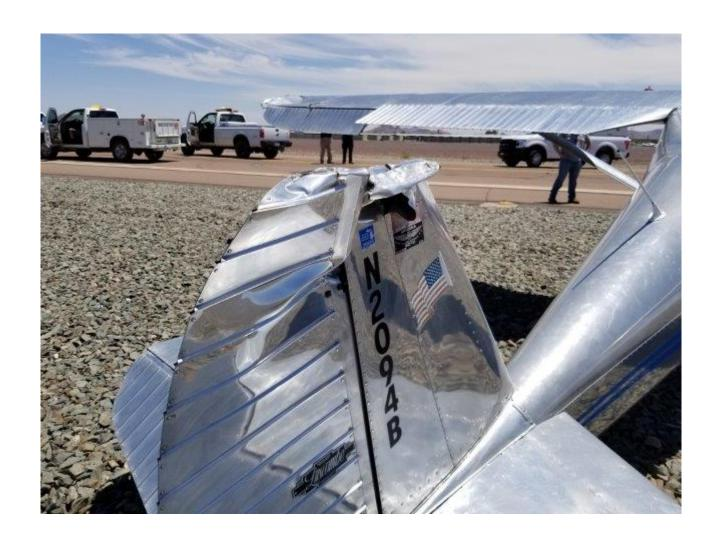
Photo 2 – View of damaged rudder (Photo courtesy of the Airport Supervisor)
