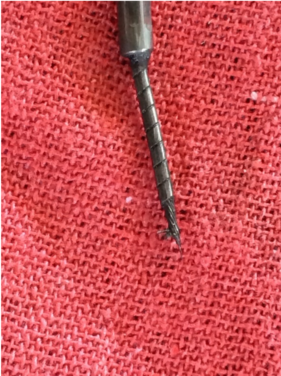
Figure 4 – Throttle Cable Separated End
