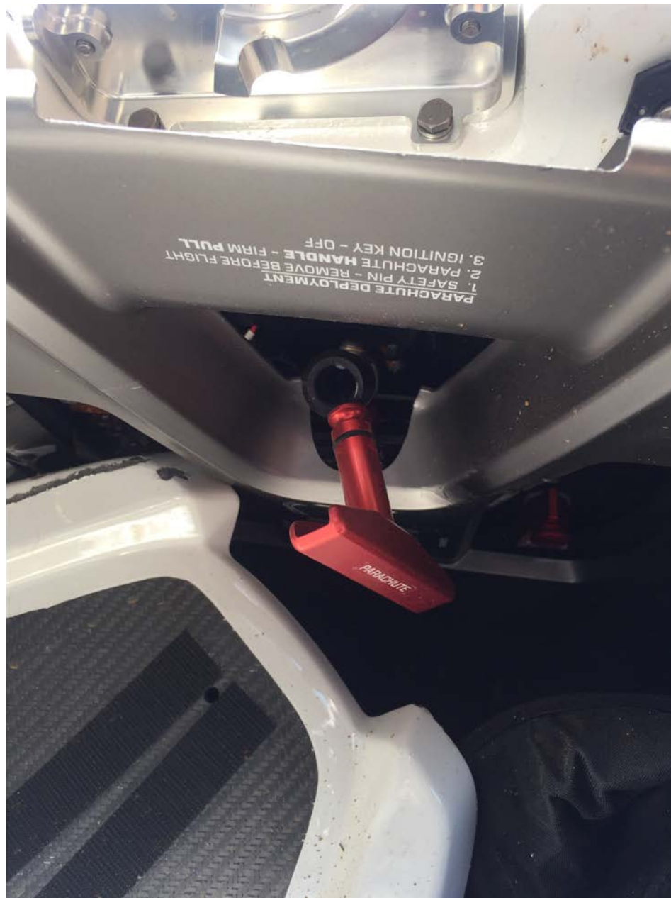
Photo 14 - Parachute Deployment Handle – At the accident site.
