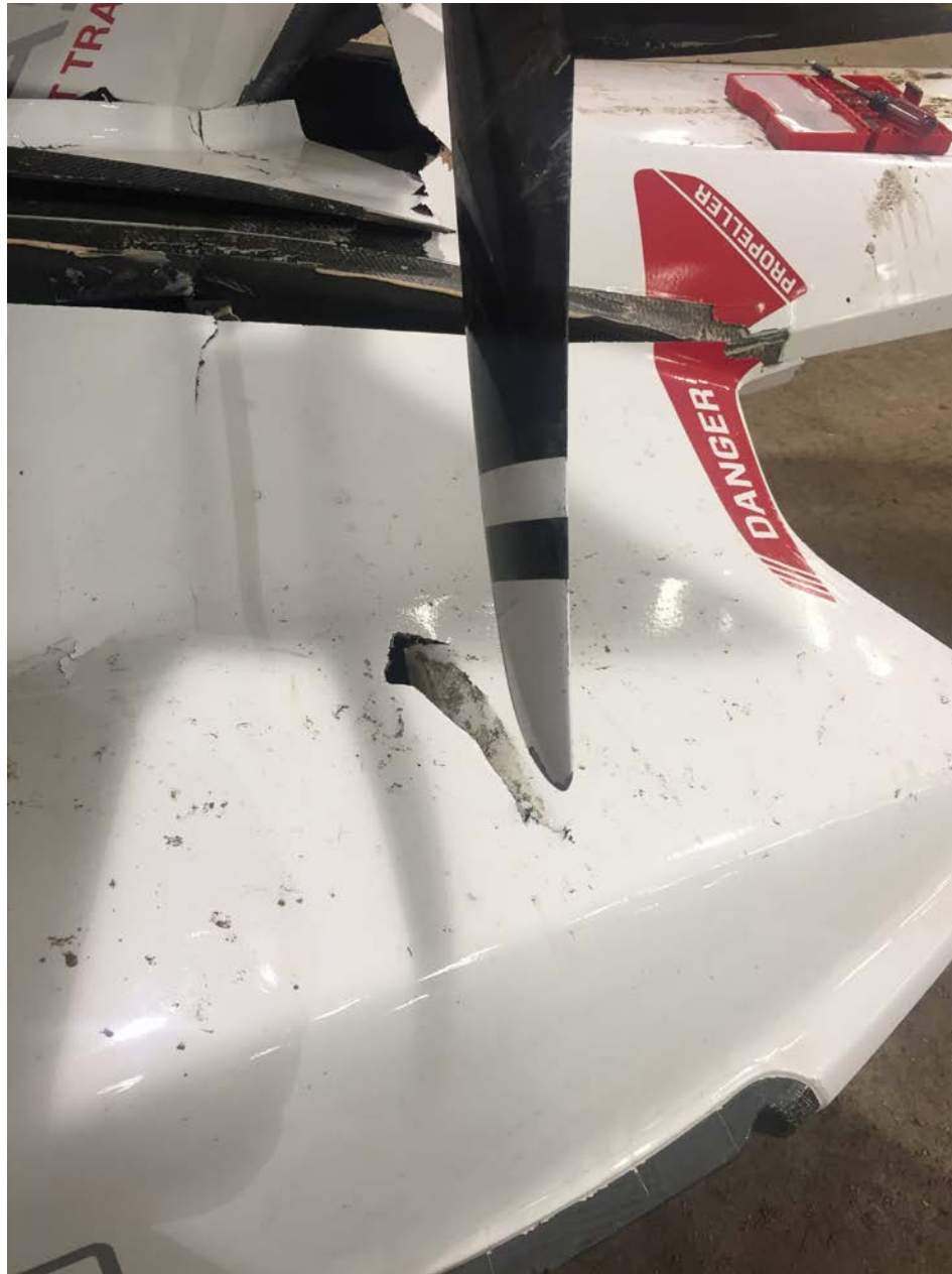
Photo 13 - View of the propeller that was embedded within the sea wing.
