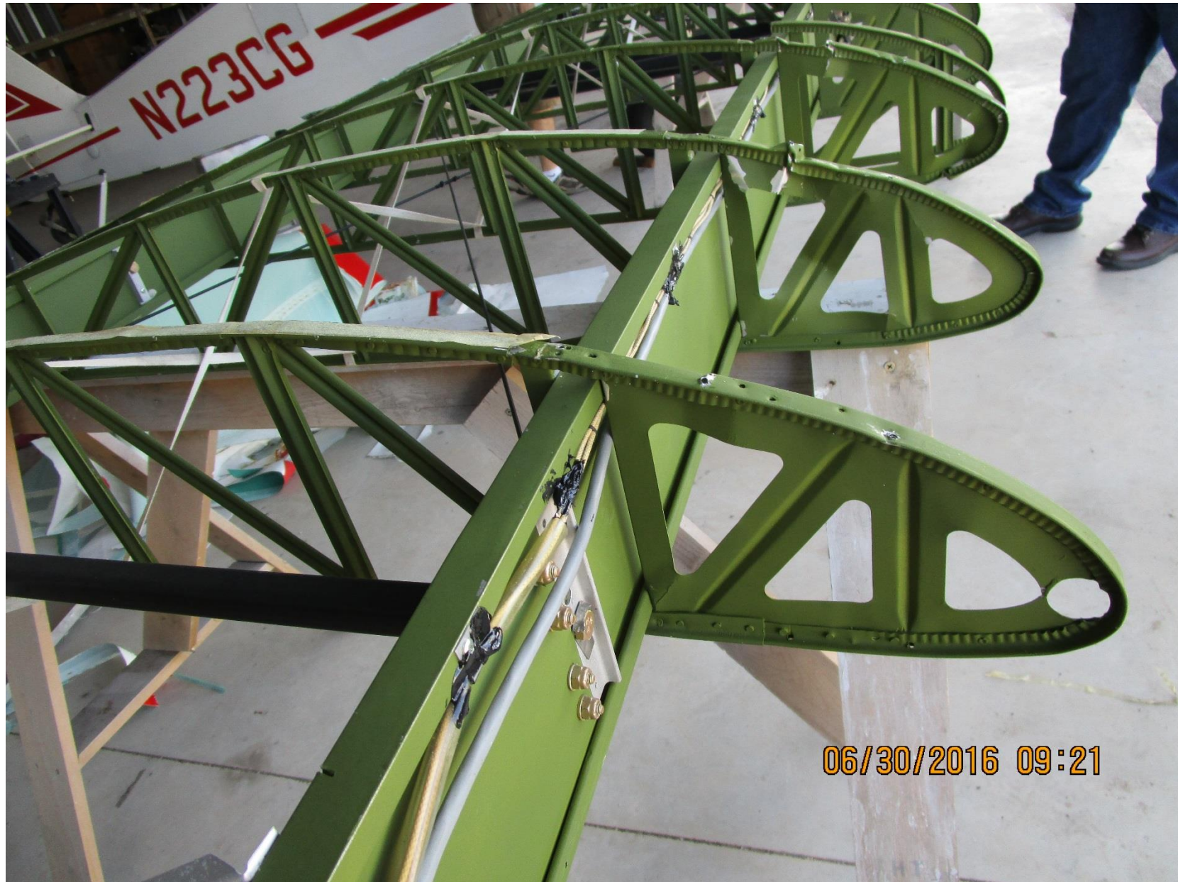
Photo 1 – View of damaged right wing ribs (photo courtesy of the FAA)
