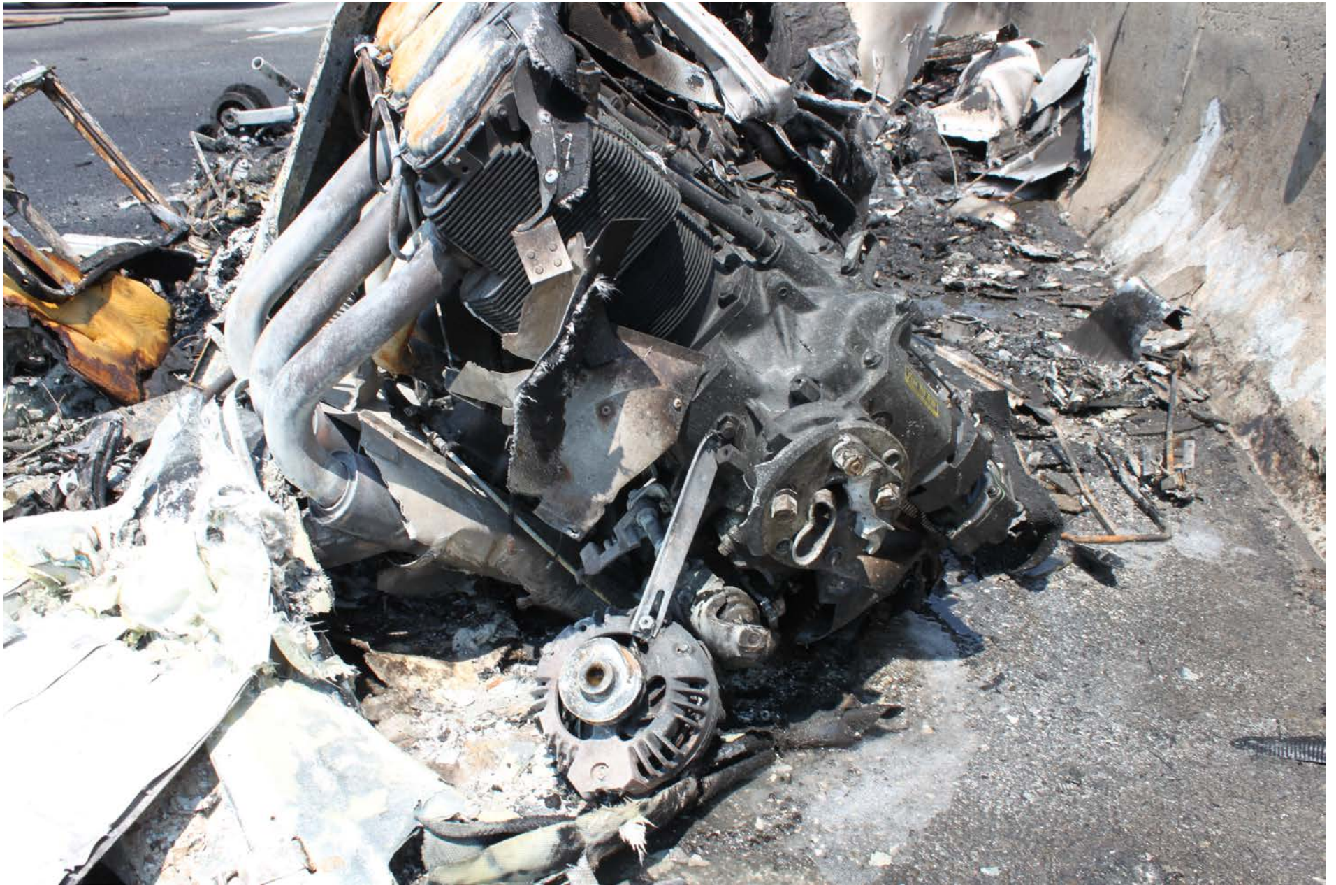
Photo 8 – Front view of engine with broken propeller flange
