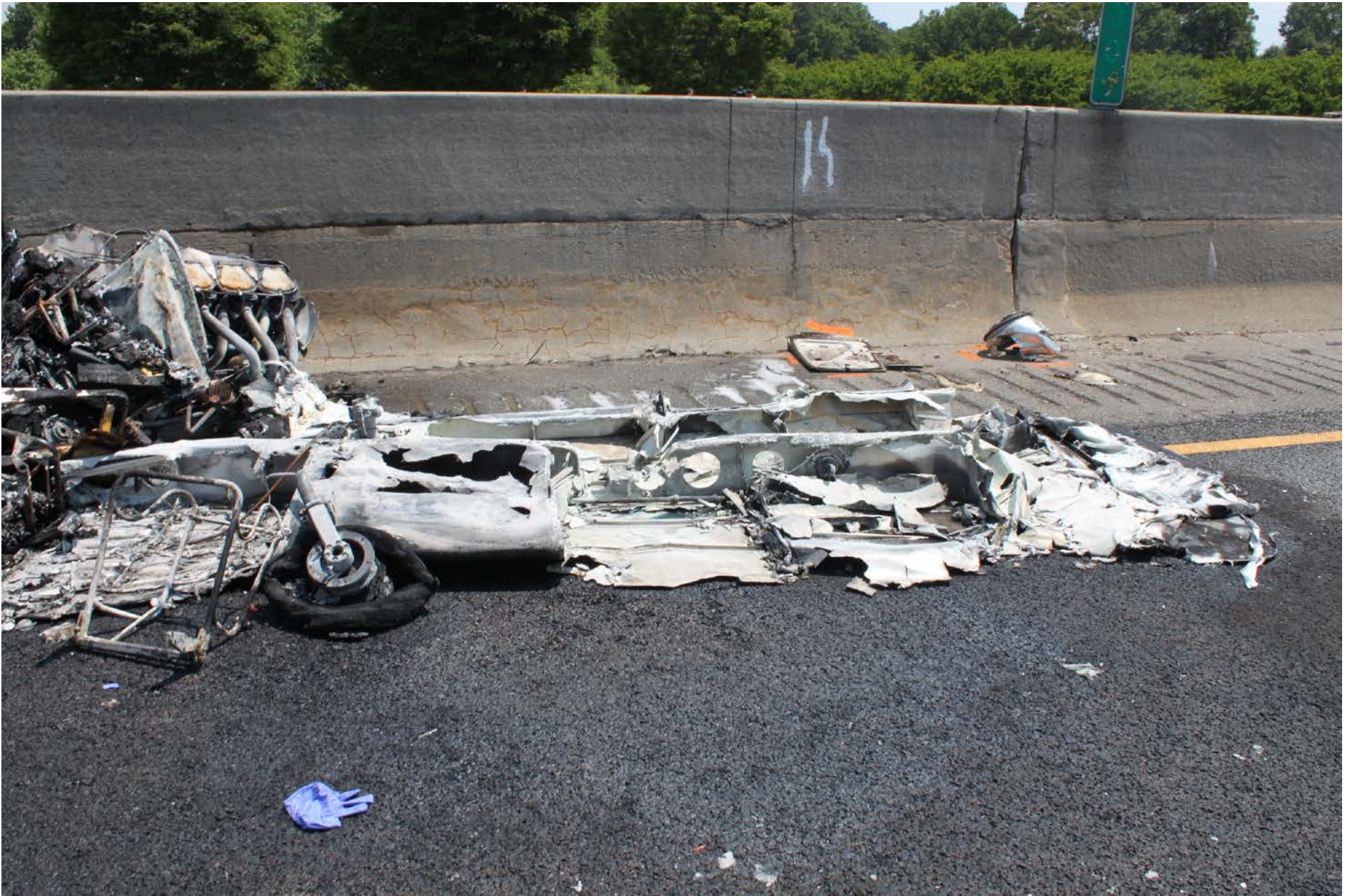
Photo 6 – View of fire damaged right wing
