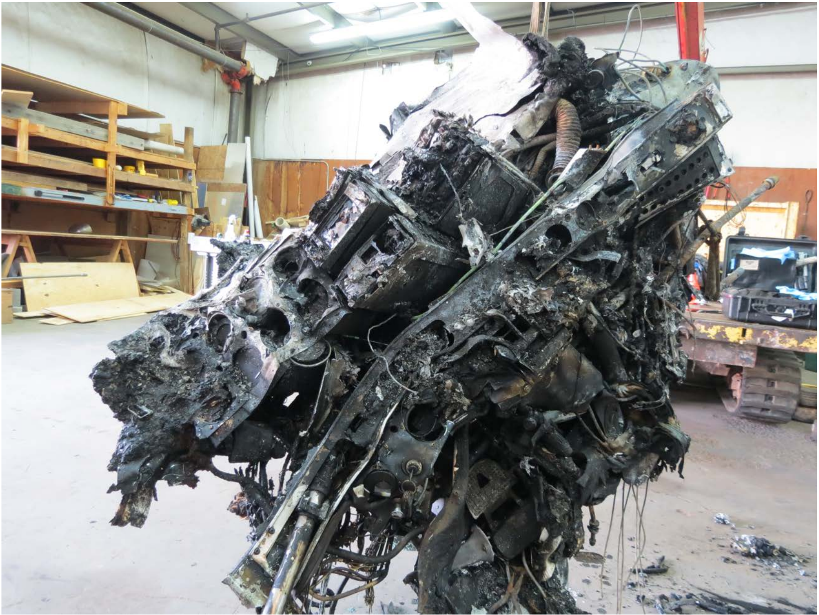
Photo 11 –View of fire damaged instrument panel
