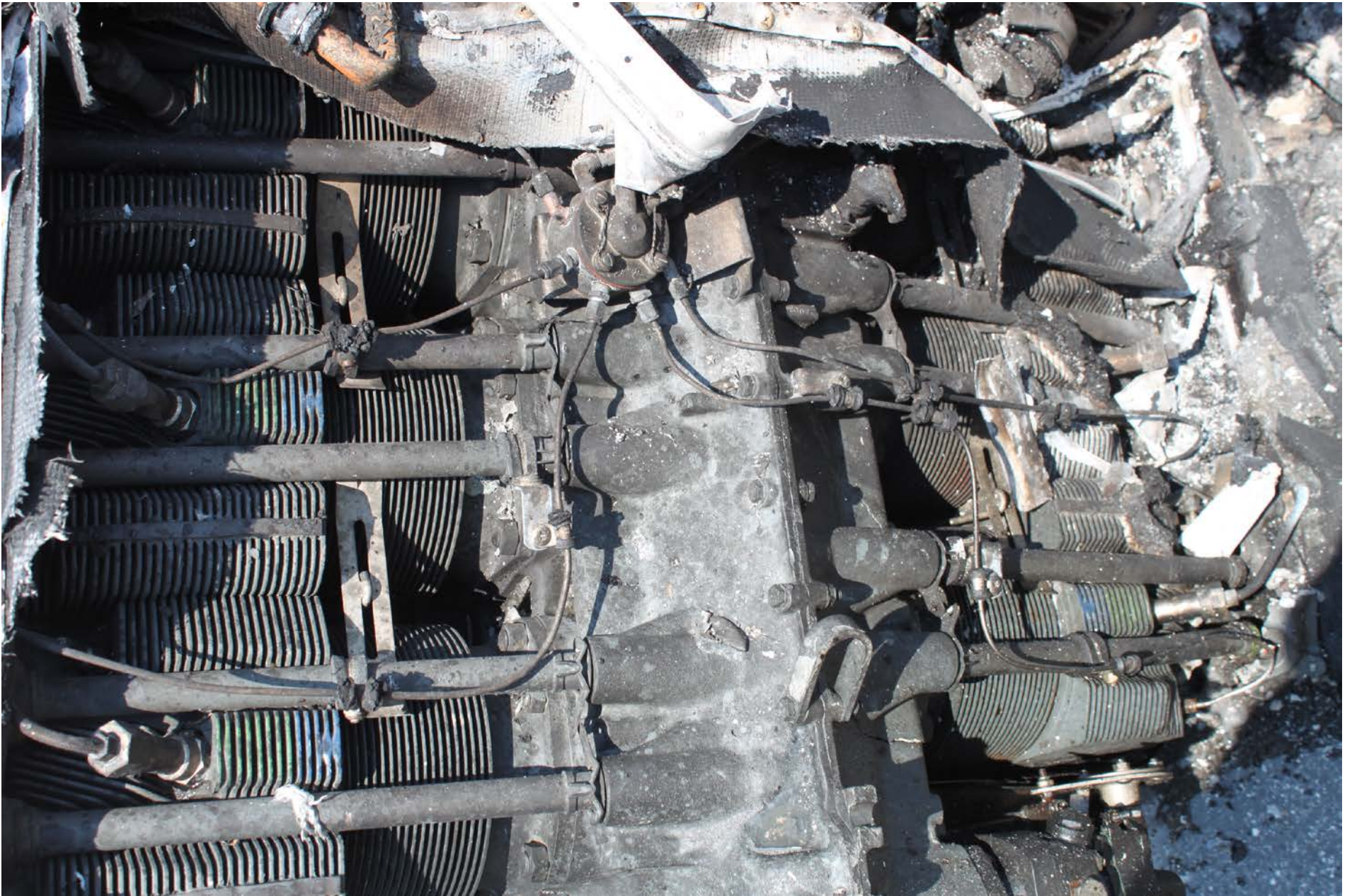
Photo 9 – View of top of engine with fuel manifold
