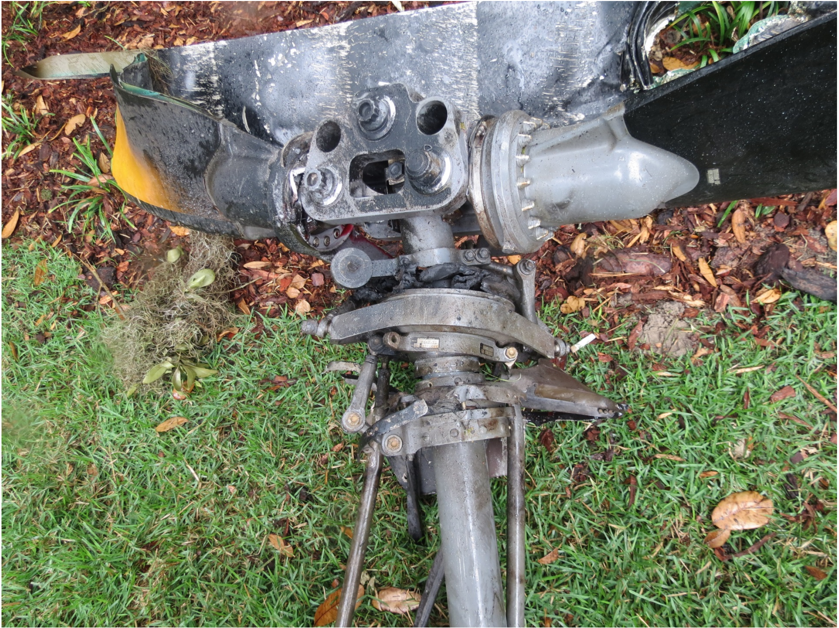
Photo 8 – View of main rotor swash plate and main rotor head
