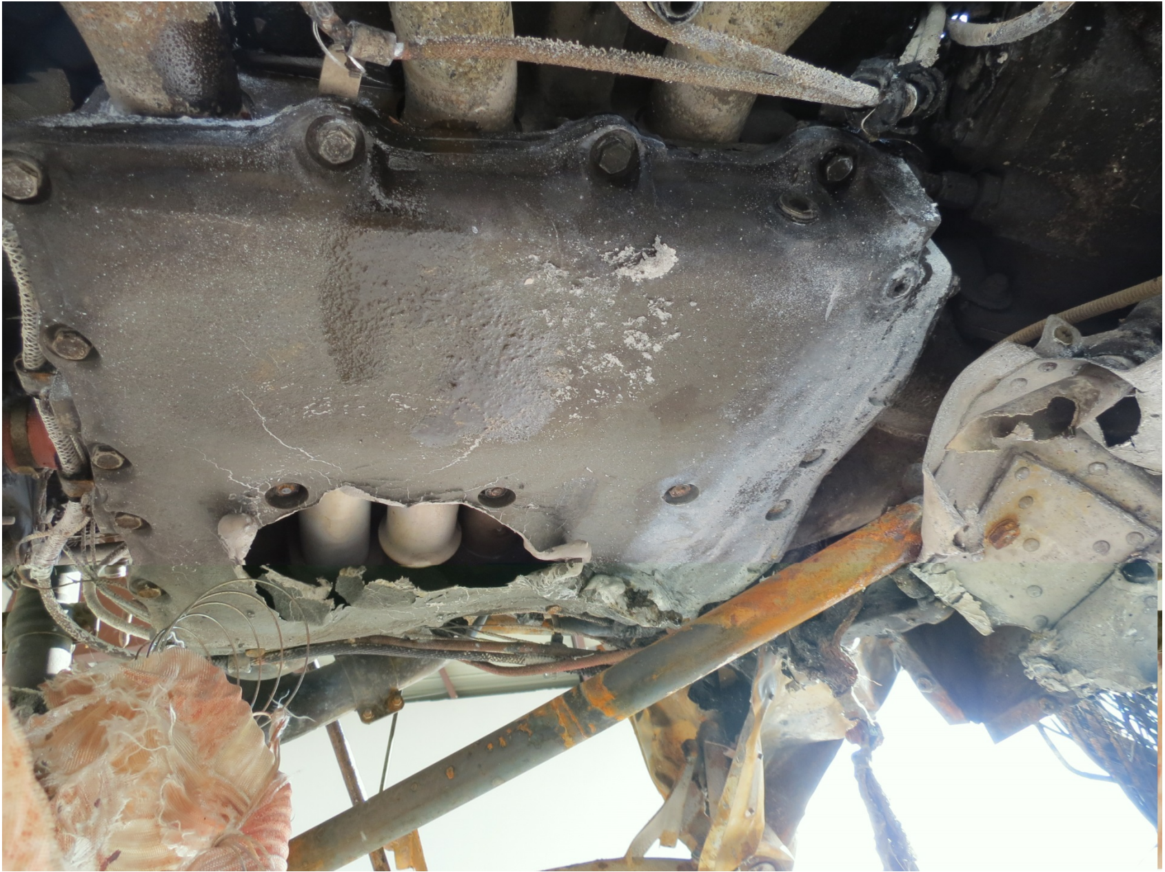
Photo 18 –View of bottom of engine showing engine sump
