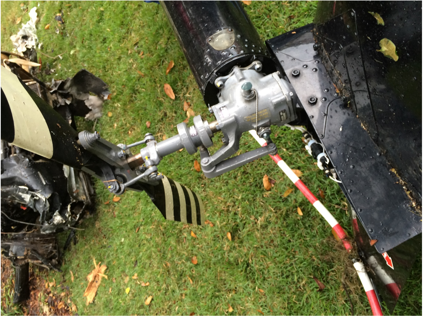
Photo 7 –View of tail rotor gear box
