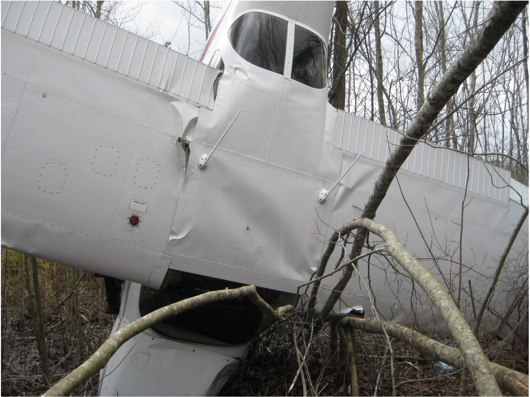
Photo 3 - View of buckled upper fuselage
