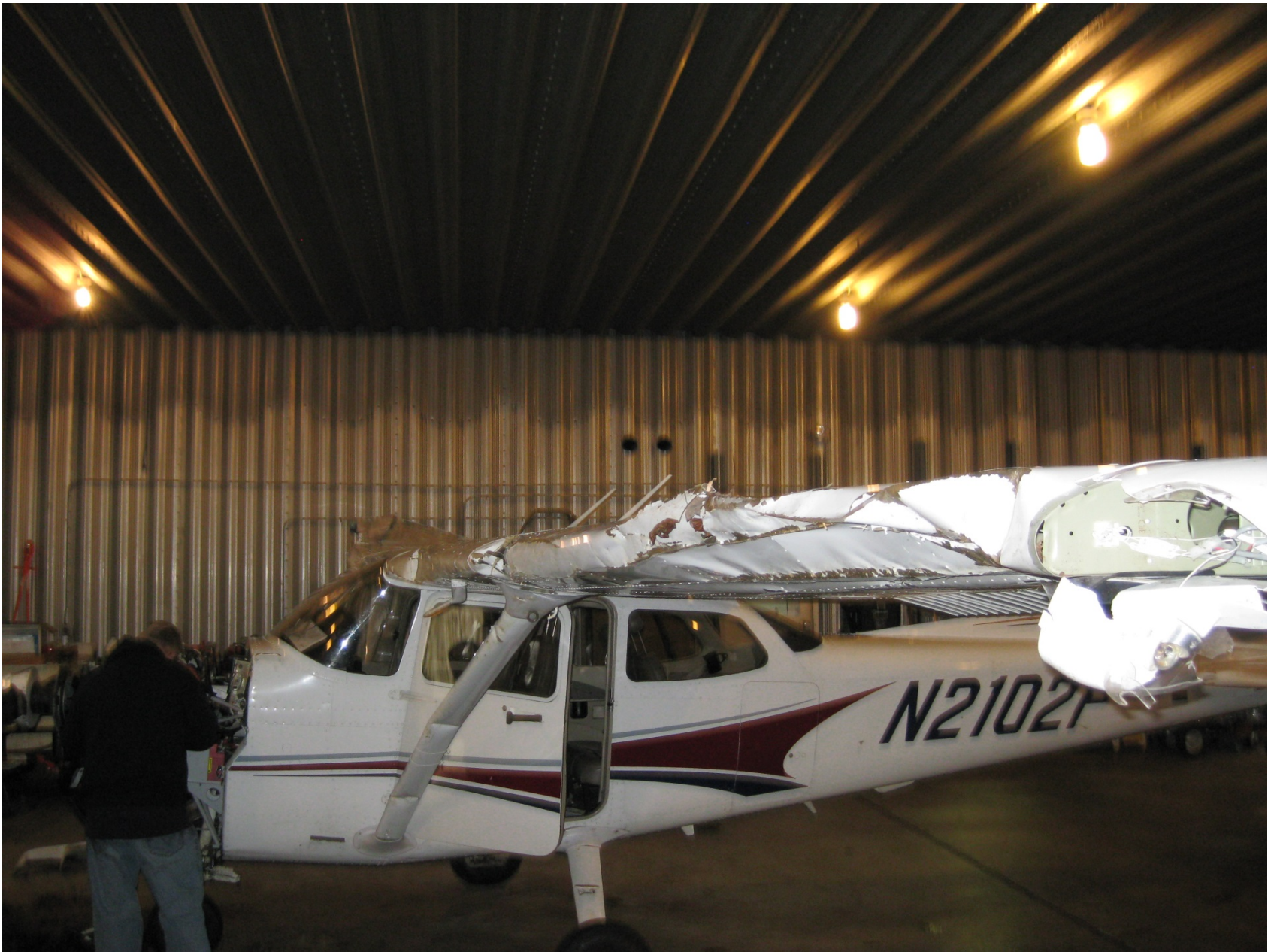
Photo 6 - View of damaged right wing
