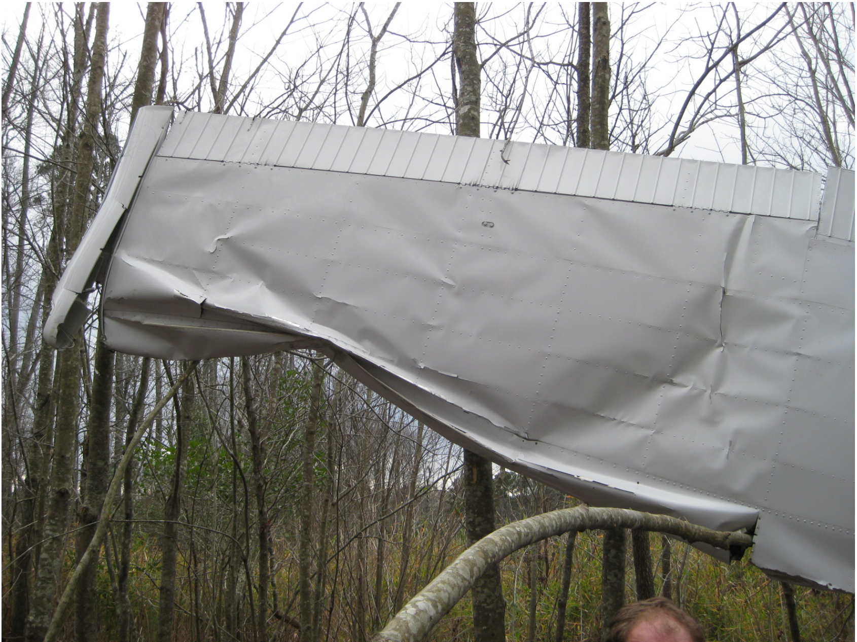
Photo 2 - View of buckled right wing leading edge
