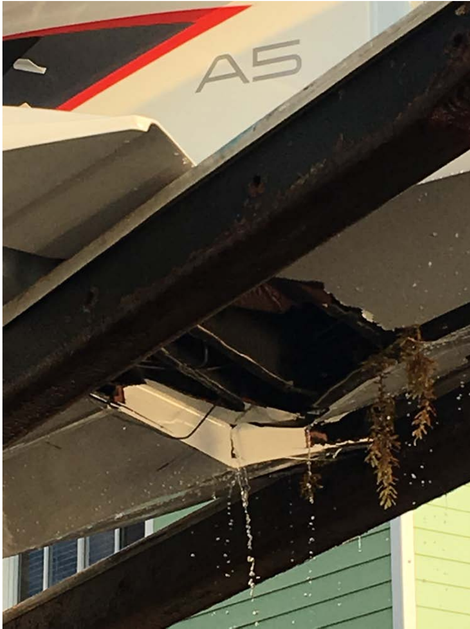
Photo 2 – View of hull damage from underneath (photo courtesy of the FAA)
