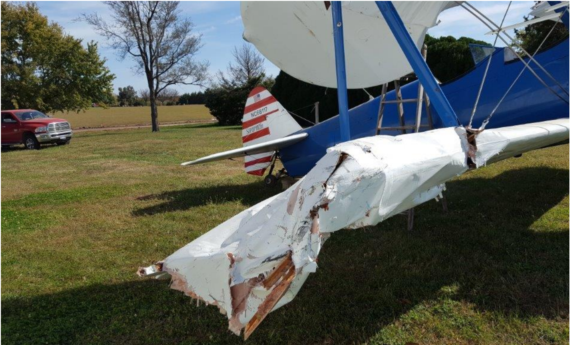
Photo 1 – View of damaged upper and lower right wings of N68117 (photo courtesy of the FAA)
