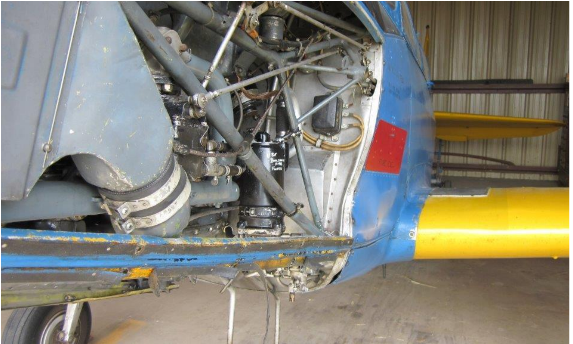
Photo 2 – View of damaged firewall of N73529 (photo courtesy of the FAA)
