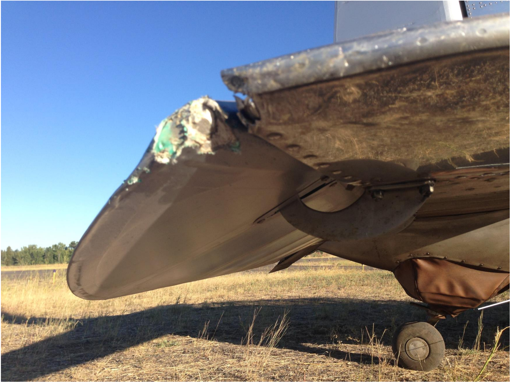
Photo 3 - Damaged elevator (Photo courtesy of the FAA)
