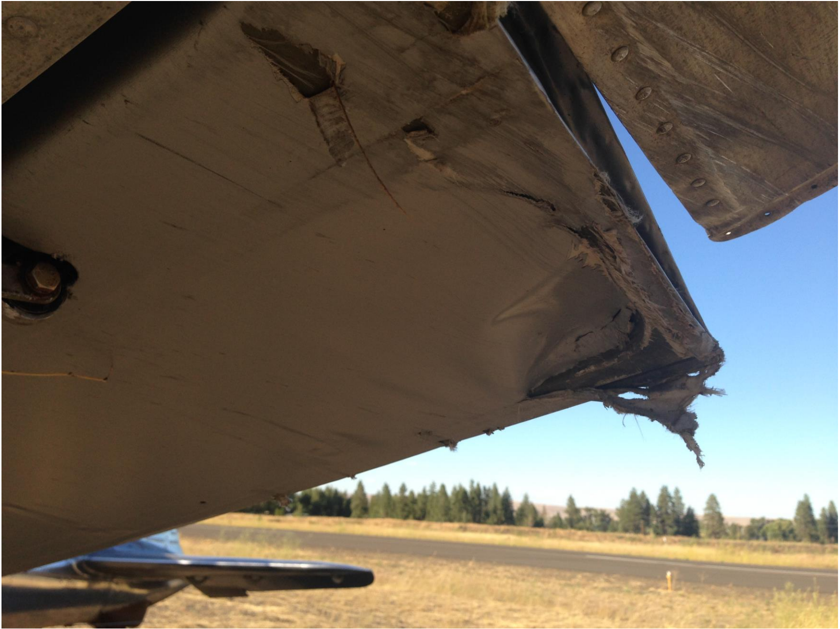
Photo 2 - Damaged left aileron (Photo courtesy of the FAA)
