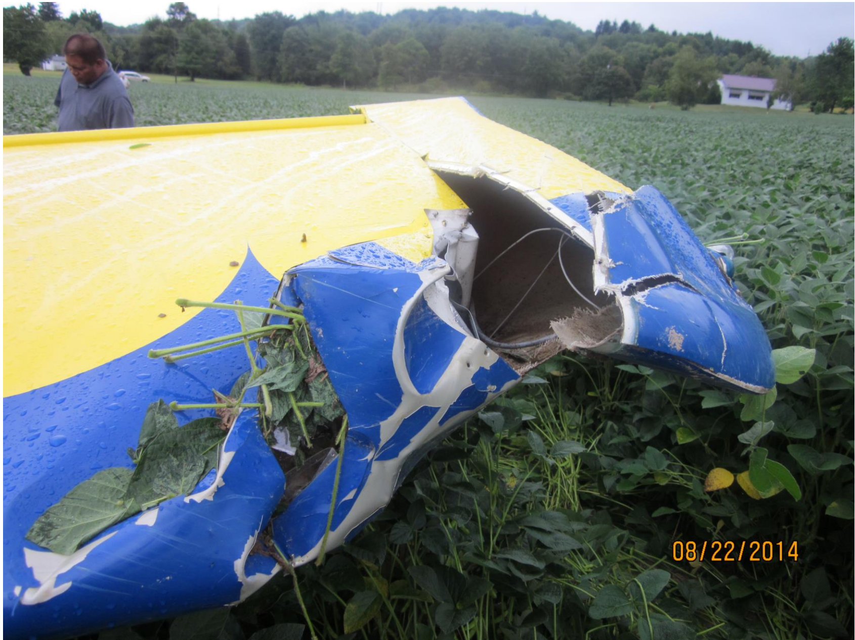
Photo 2 – Right Wing Damage (Courtesy of FAA)
