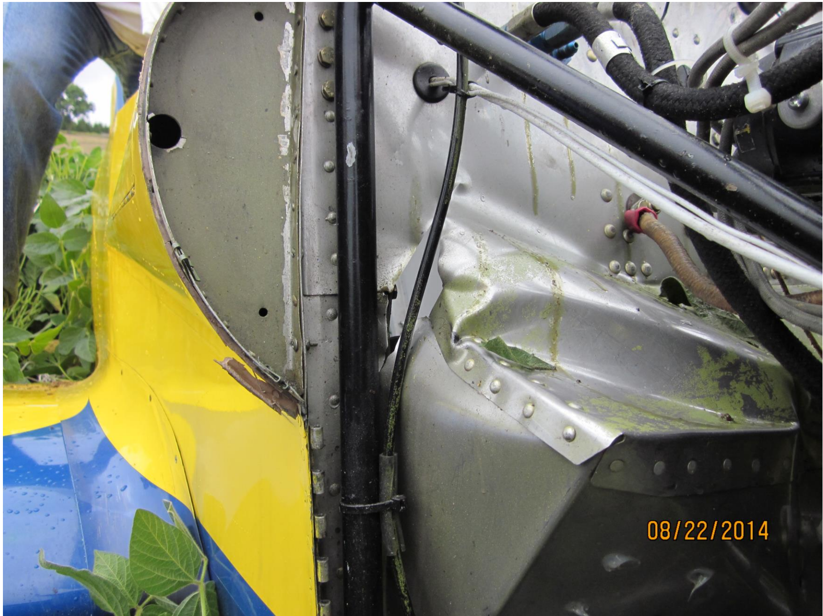
Photo 3 – Firewall Damage (Courtesy of FAA)
